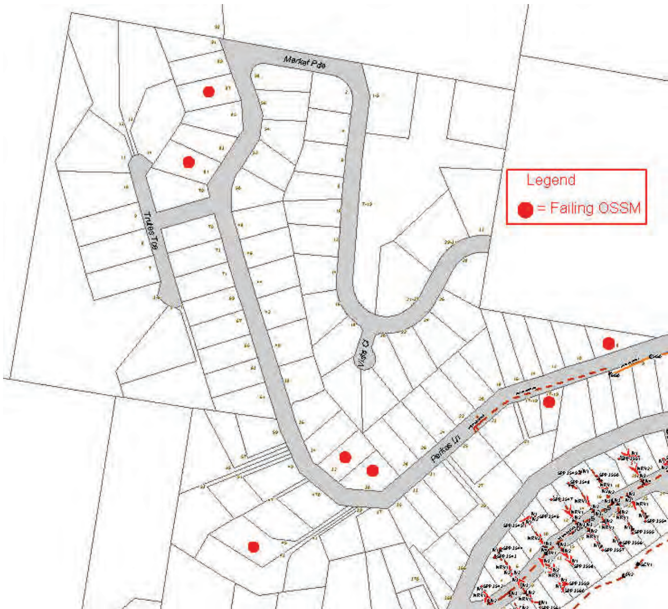
Location of Failing OSSMs in Parkes Lane.
