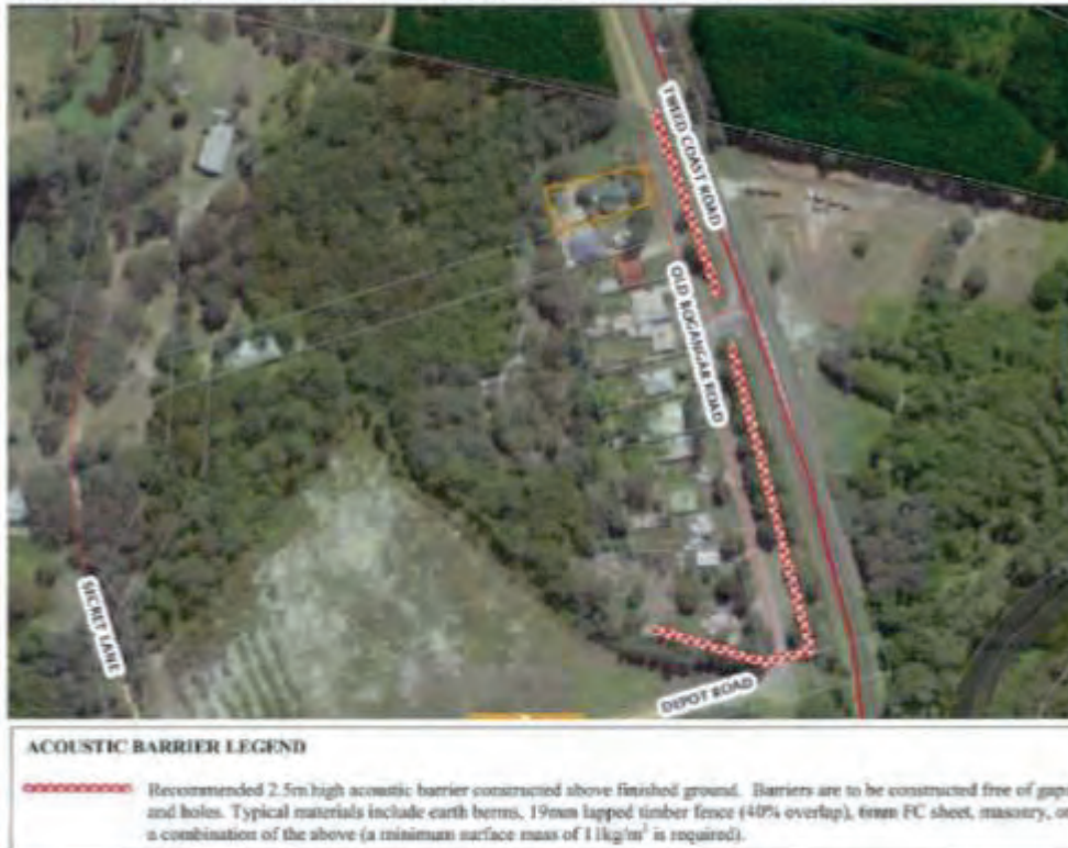
Sketch No. 2: Tweed Coast Road Existing Dwellings and Recommended Acoustic Barriers (Not to Scale)
