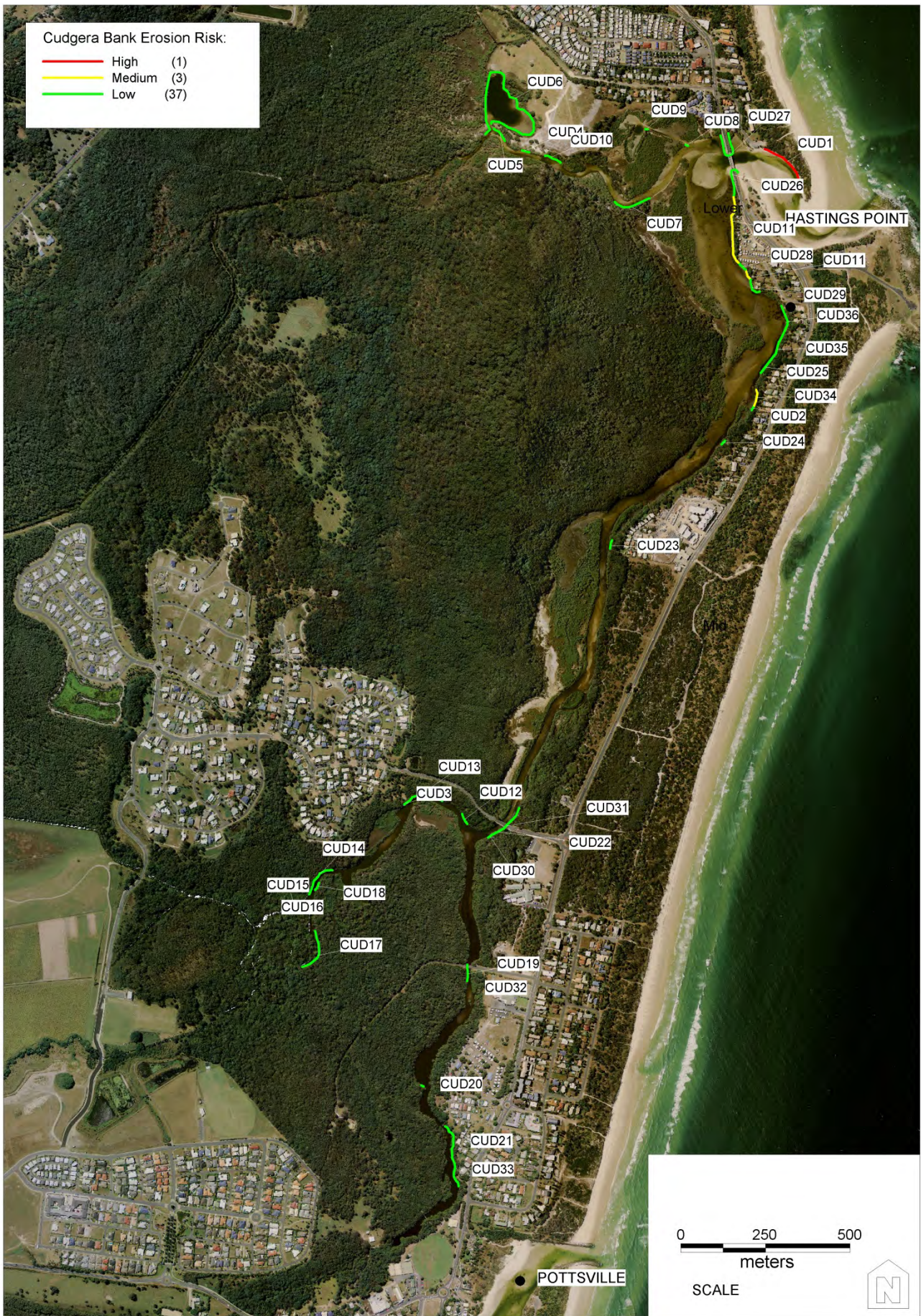
Figure 21: Cudgera Creek Bank Erosion Risk (refer Appendix 3 for further details)
