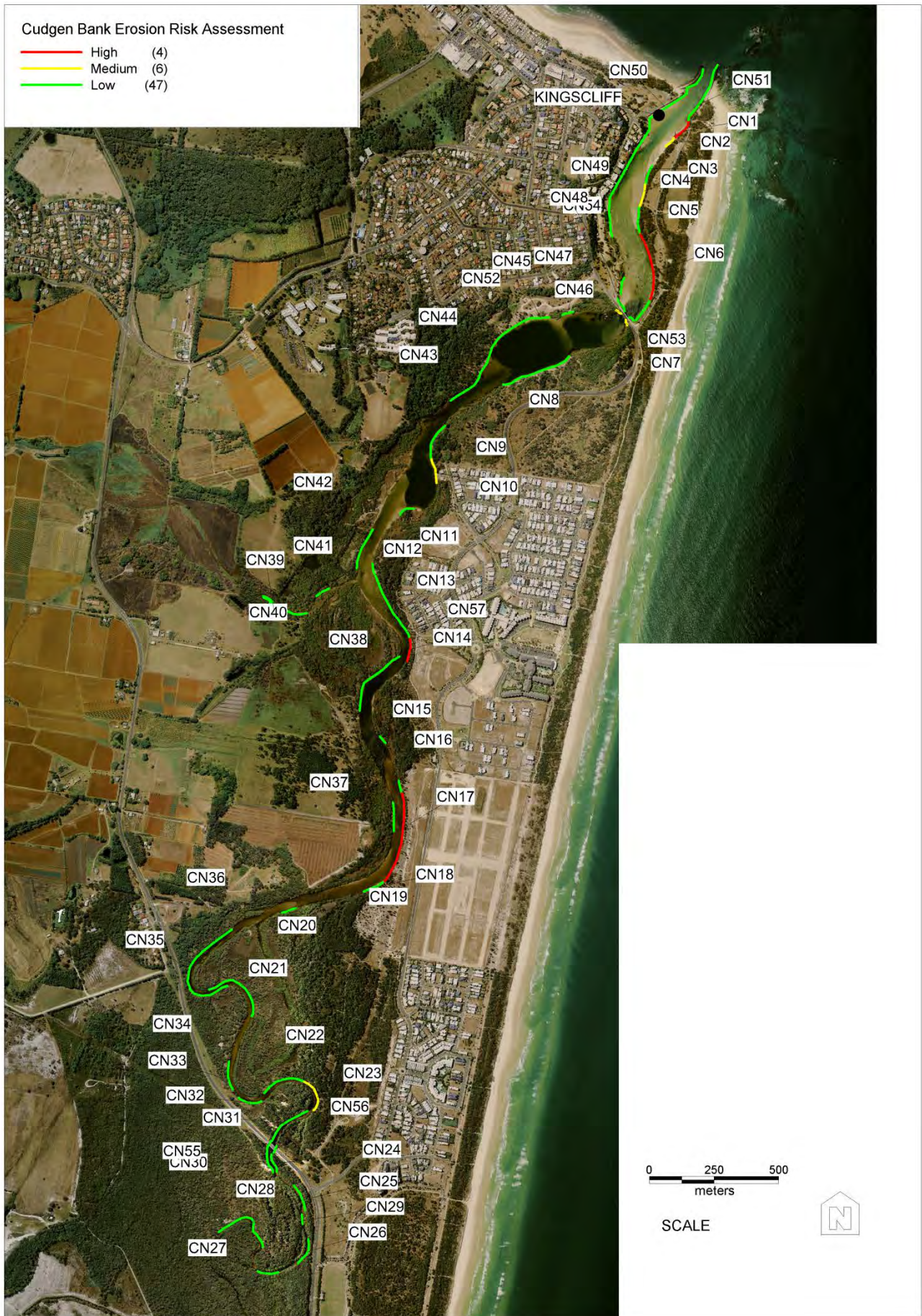
Figure 20: Cudgen Creek Bank Erosion Risk (refer Appendix 3 for further details)
