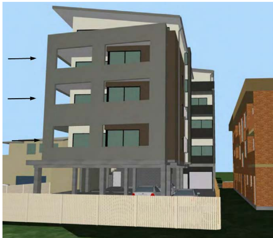
Figure 4: Location of balconies which feature a 2m side setback at northern side boundary (adjoining commercial 2 storey commercial building)
