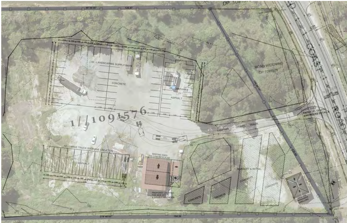
Figure 3: Proposed plan transposed over aerial imagery (source: Extract from submitted DA Plans and Aerial Image extracted from TSC GIS, weave)*
