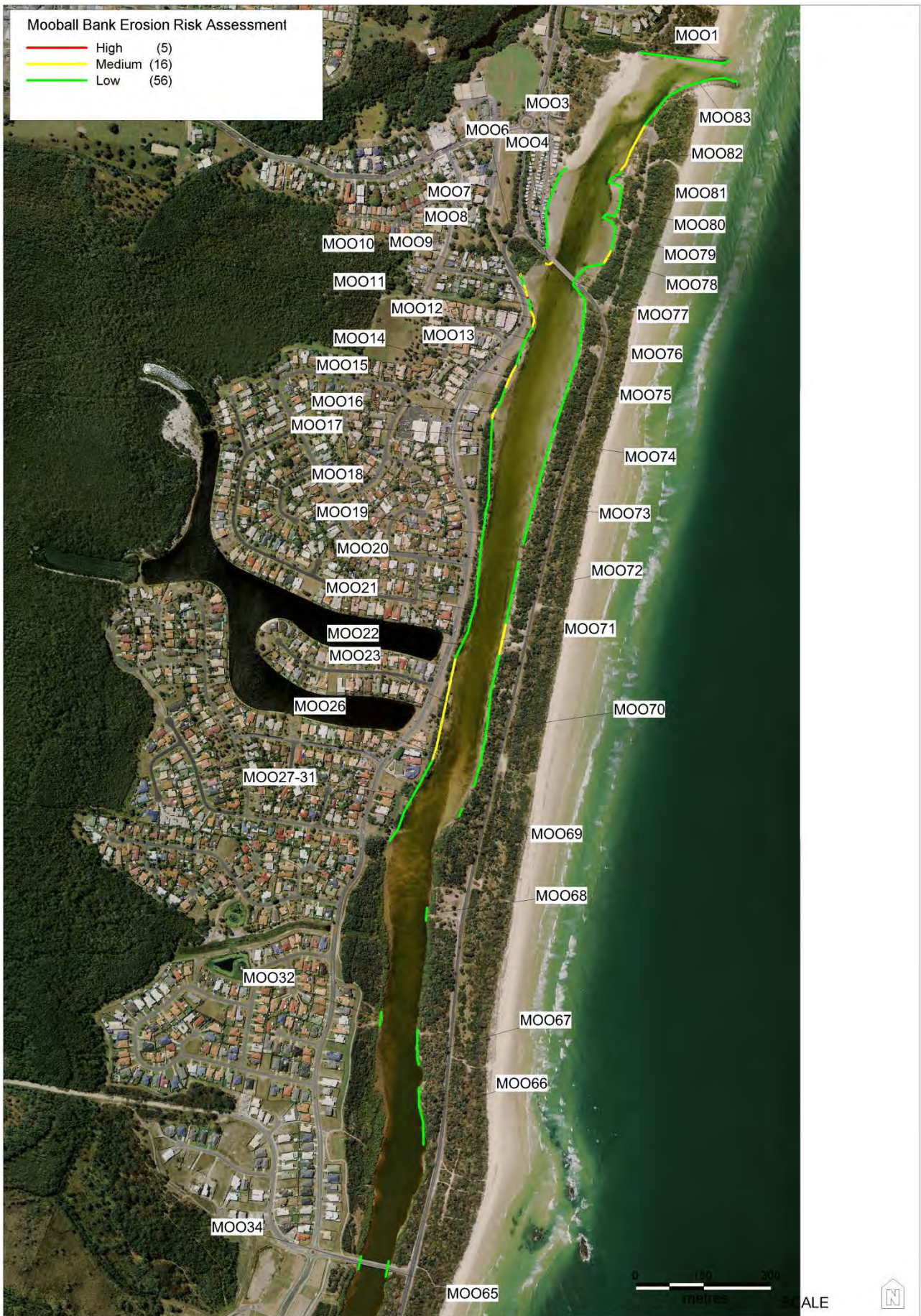
Figure 22: Mooball Creek Bank Erosion Risk (refer Appendix 3 for further details)
