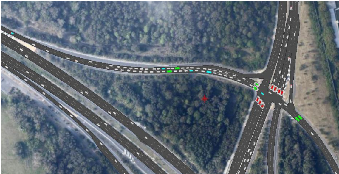
Figure 4.4: Southbound Queuing at Tugun Bypass off-ramp
