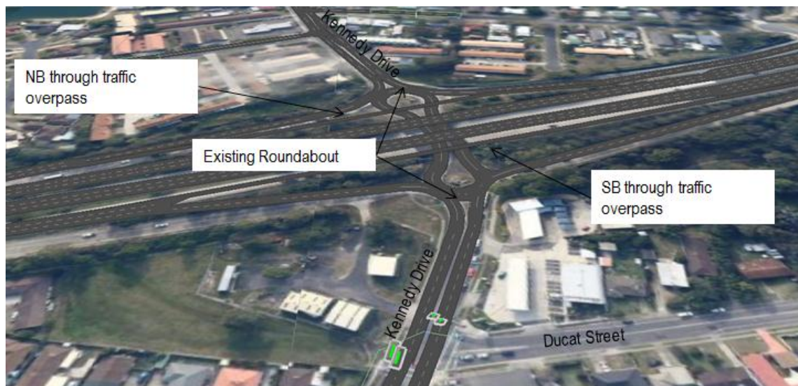
Figure 2.9: Planned Through Traffic Overpass for Kennedy Drive
