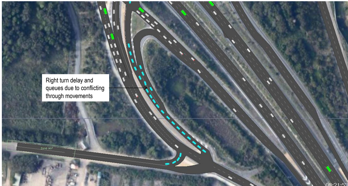
Figure 4.2: Priority Controlled Intersection Failure with Development Traffic – AM Peak
