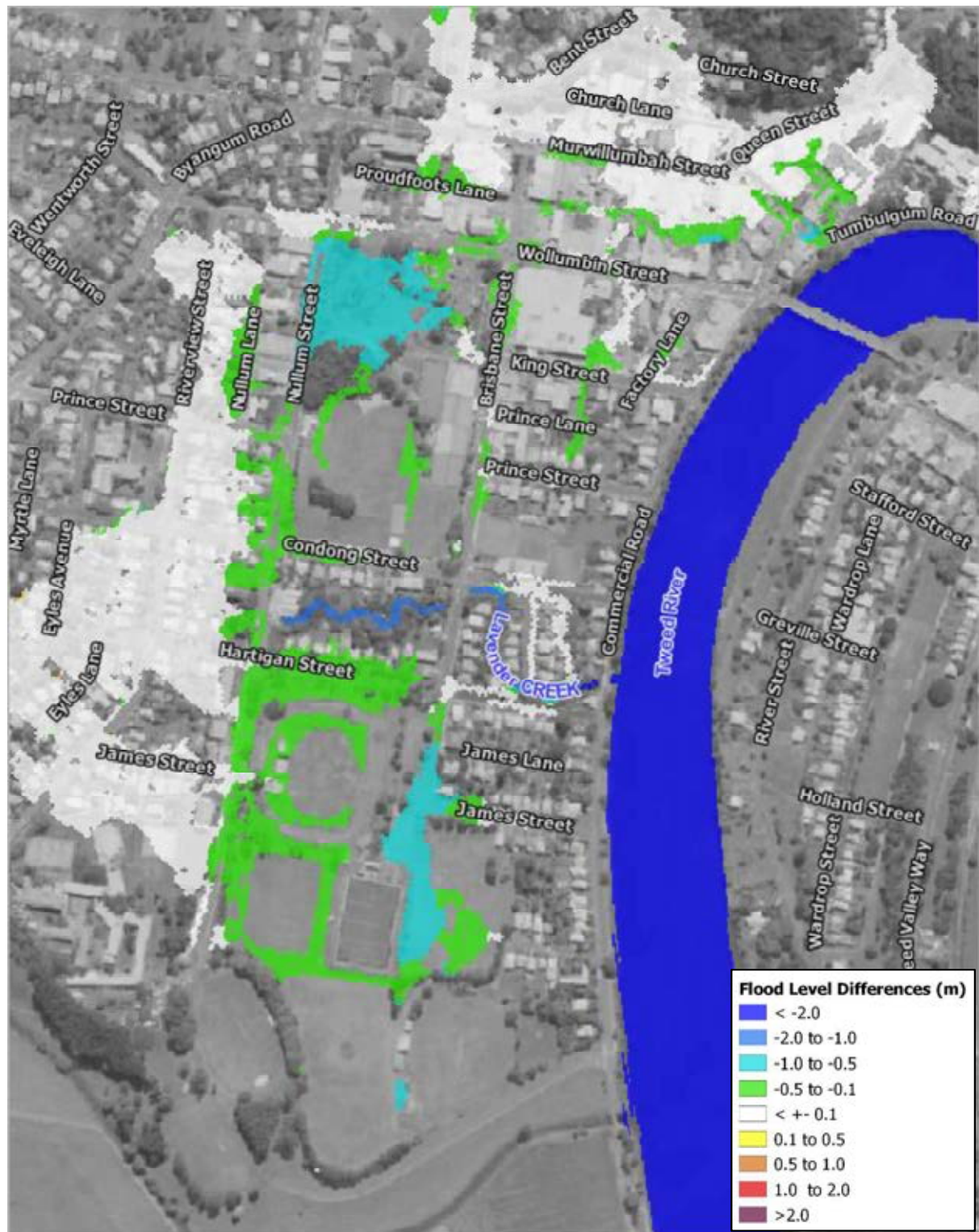
Predicted change in 20% AEP water levels across the Murwillumbah CBD with a low Tweed River water level
