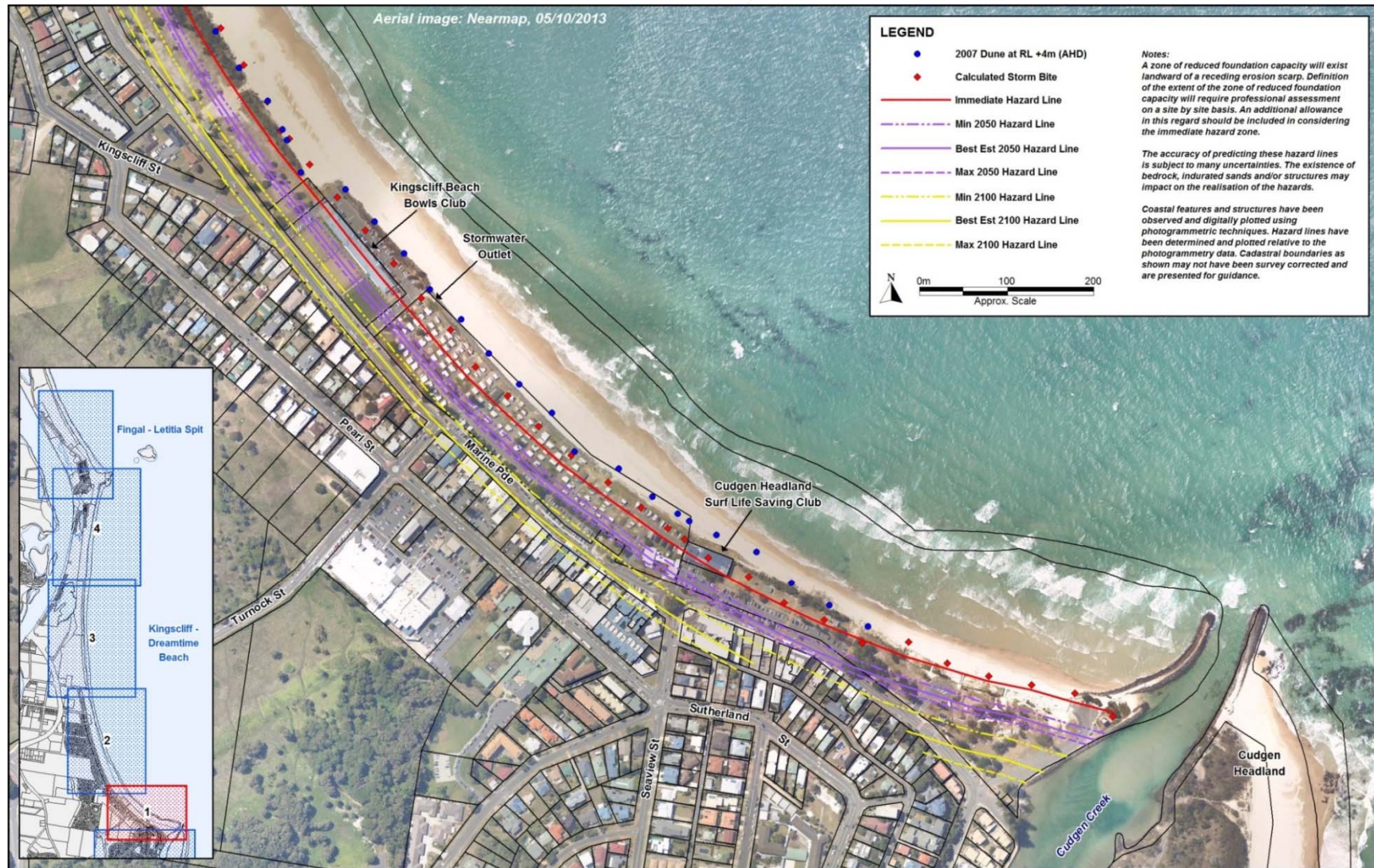
Figure 2-3 Erosion Hazard Zones: Kingscliff
