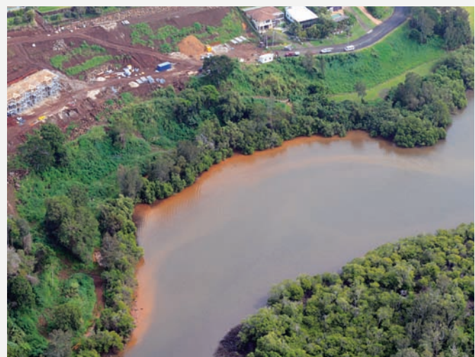
Sediment runoff from adjacent land development.
