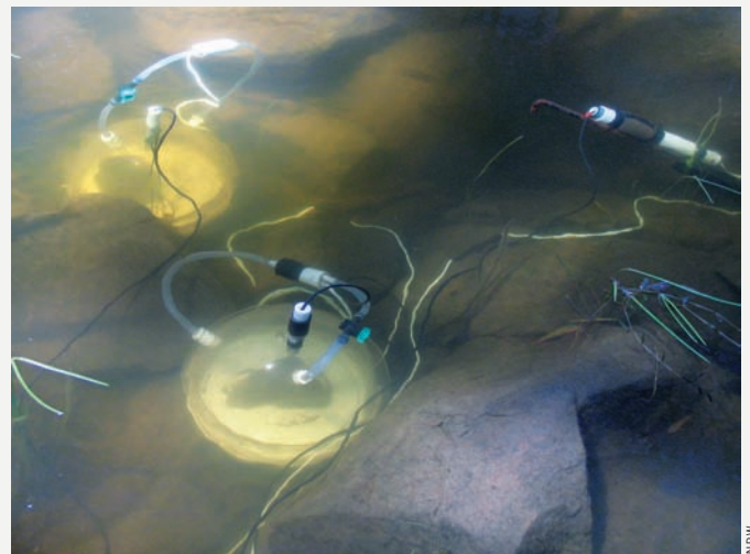
Benthic respiration and gross primary productivity are measured using plastic, dome shaped chambers placed on the stream bed.
