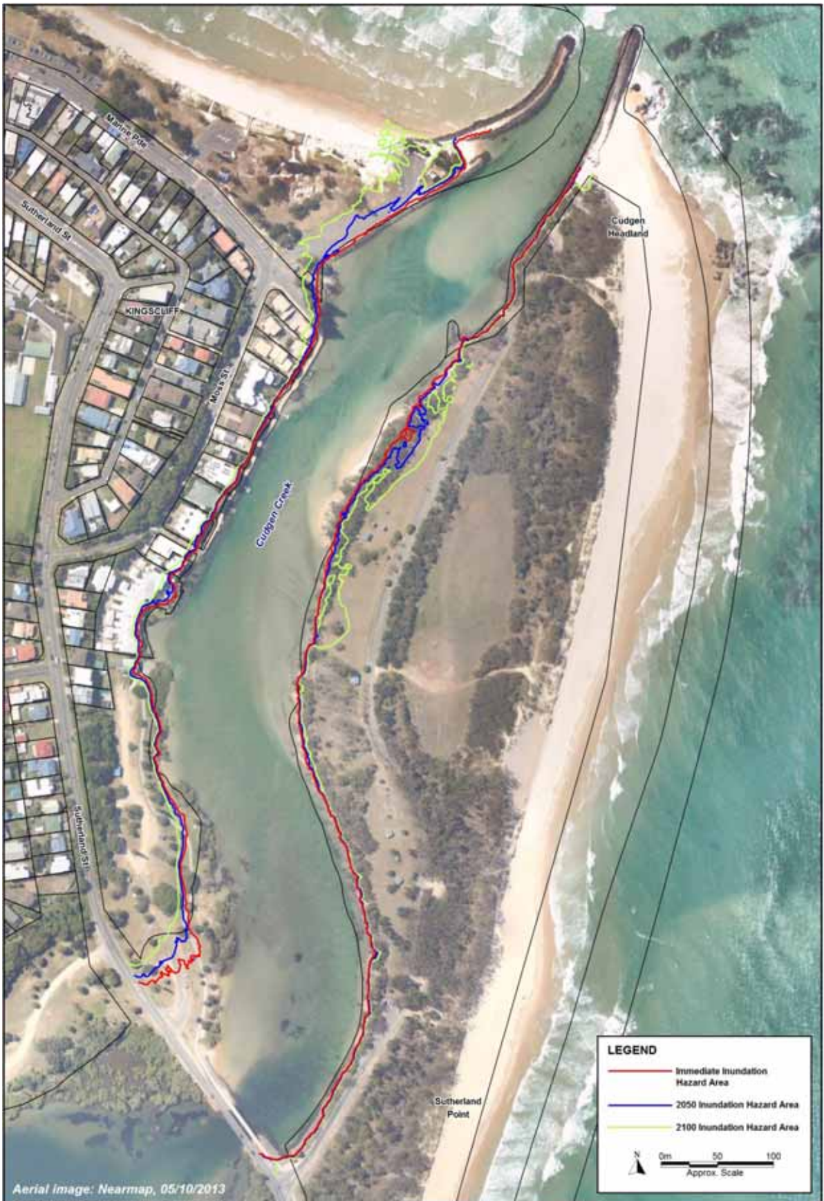
Figure 4-14 Cudgen Creek lower estuary inundation hazard zones
