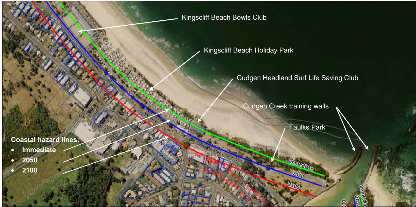
Figure 3 - Kingscliff Coastal Hazard Lines (Immediate, 2050 and 2100) overlaid on aerial image of the area (image courtesy of Tweed Shire Council), based on updated calculation (WRL, 2010).
