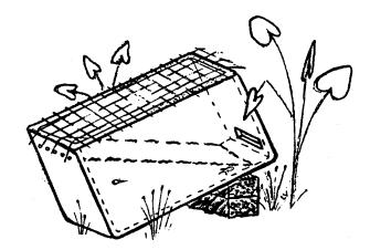
A polystyrene broccoli box for raising very young tadpoles out of reach of fish. Use dam water and no more than one spawn clump per box. Note the wire mesh lid against predators and the overflow holes. The slope allows for up to twenty tadpoles to be retained in the box until they turn into frogs, without them drowning. If there is a slit in the box, level with the top of the land area, and if the box is placed adjacent to the dam, then the young frogs can leave the box when they are ready.
