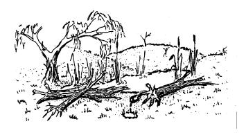
Here fallen trees protect the walls and spillway of a dam against erosion by livestock and protect at the same time a frog habitat. A wide but screened overflow pipe just below the spillway will reduce tadpole losses and spillway erosion. Non-clogging screening is achieved by attaching a full length of perforated agricultural pipe (with the far end closed off) to the pipe's intake side.
