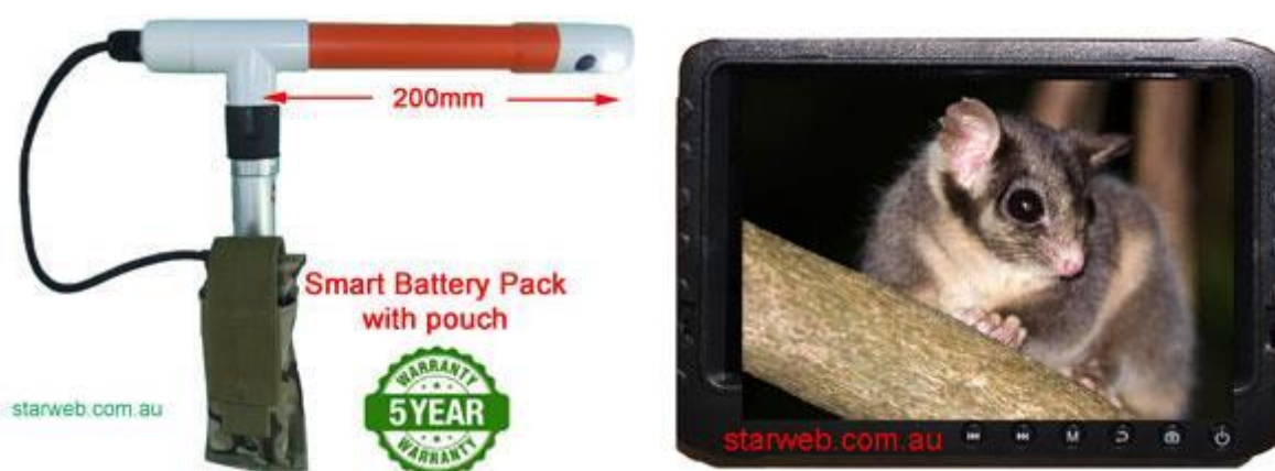
Figure 1. The camera (left) attached to the 9m pole and inserted into the hollow transmitted the image from inside the box to the handheld screen (right).
