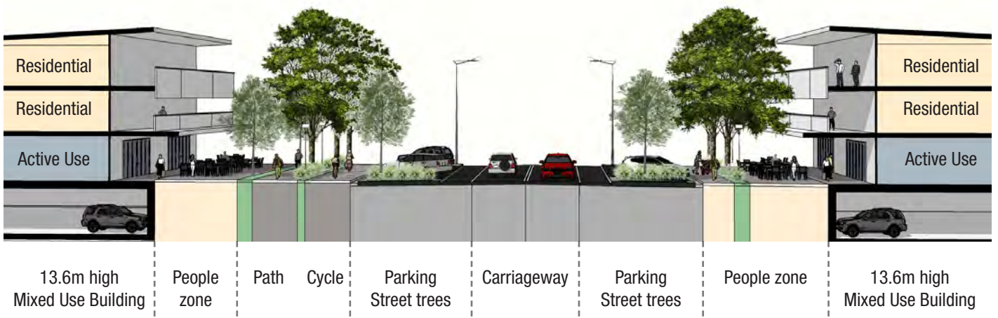
Figure 8.11 Indicative Turnock Street Section – Mixed Use Interface
