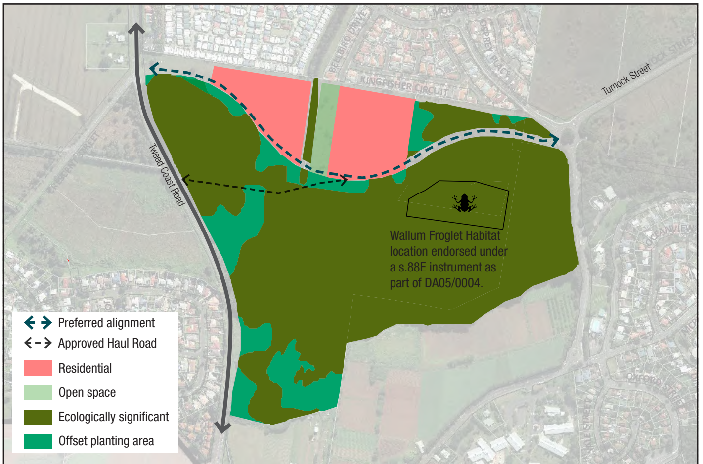
Figure 8.27 Indicative Turnock Street extension alignment option. Detailed design including intersection type and location, final road alignment, road pavement design and cross sections including fill levels, batters, drainage, integration of shared pathways will be subject to a separate a more detailed design review and approvals process.
