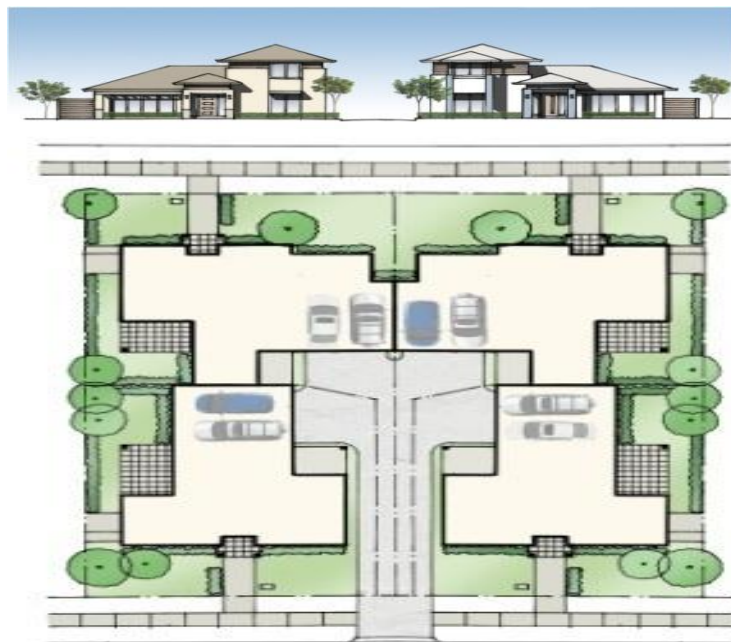
Figure 3.3.7 1 Mews dwellings (2 - 6 dwellings on one site with separate titles sharing a common driveway which might be created by either reciprocal easements or common property)
