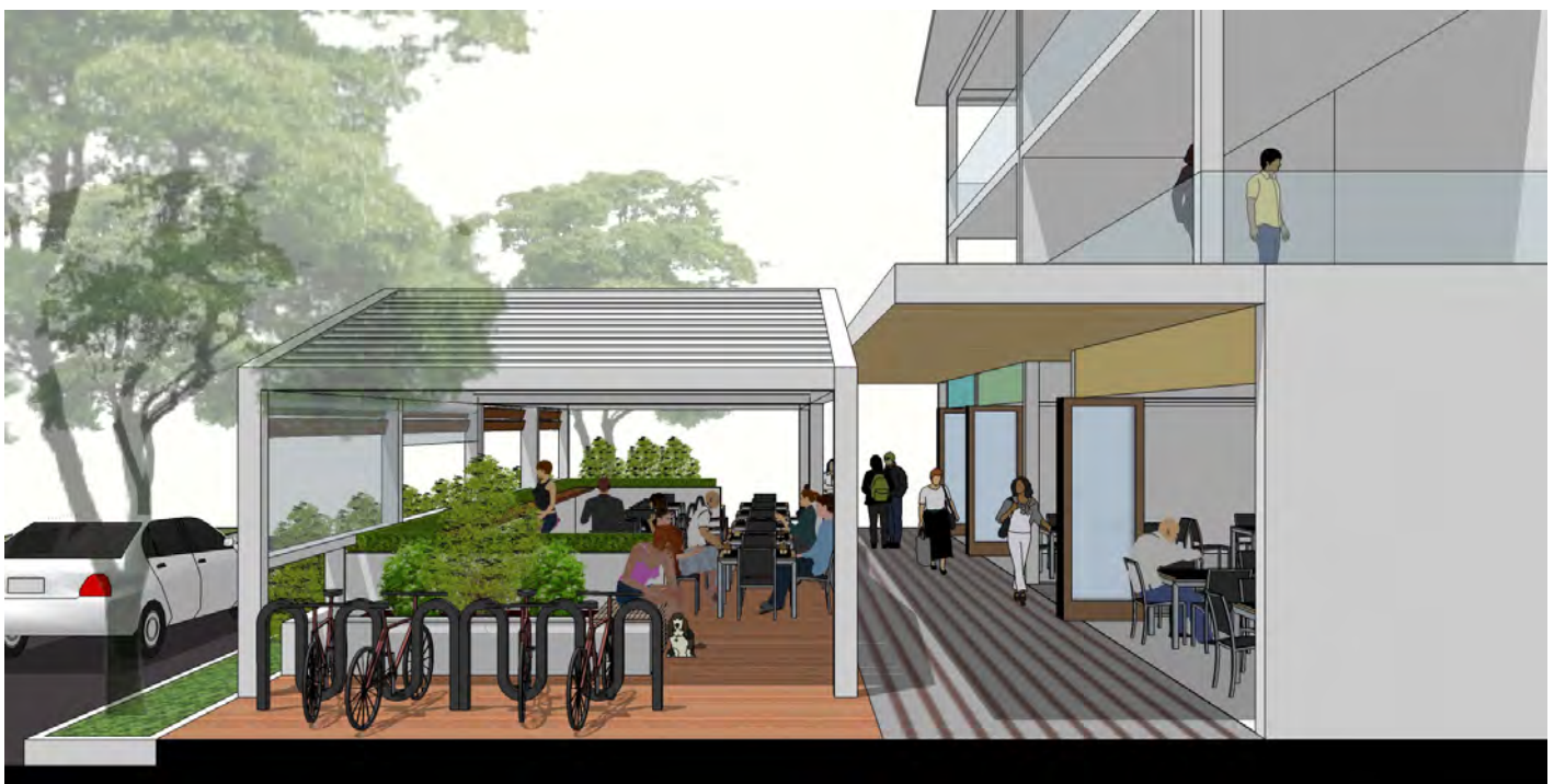
Figure 3.24 Outdoor dining areas – Design outdoor dining areas to achieve universal access and a balance between rain, wind and UV protection, shade and filtered light. Use a mix of marine tolerant materials and integrate landscaping, street furniture and bike parking.
