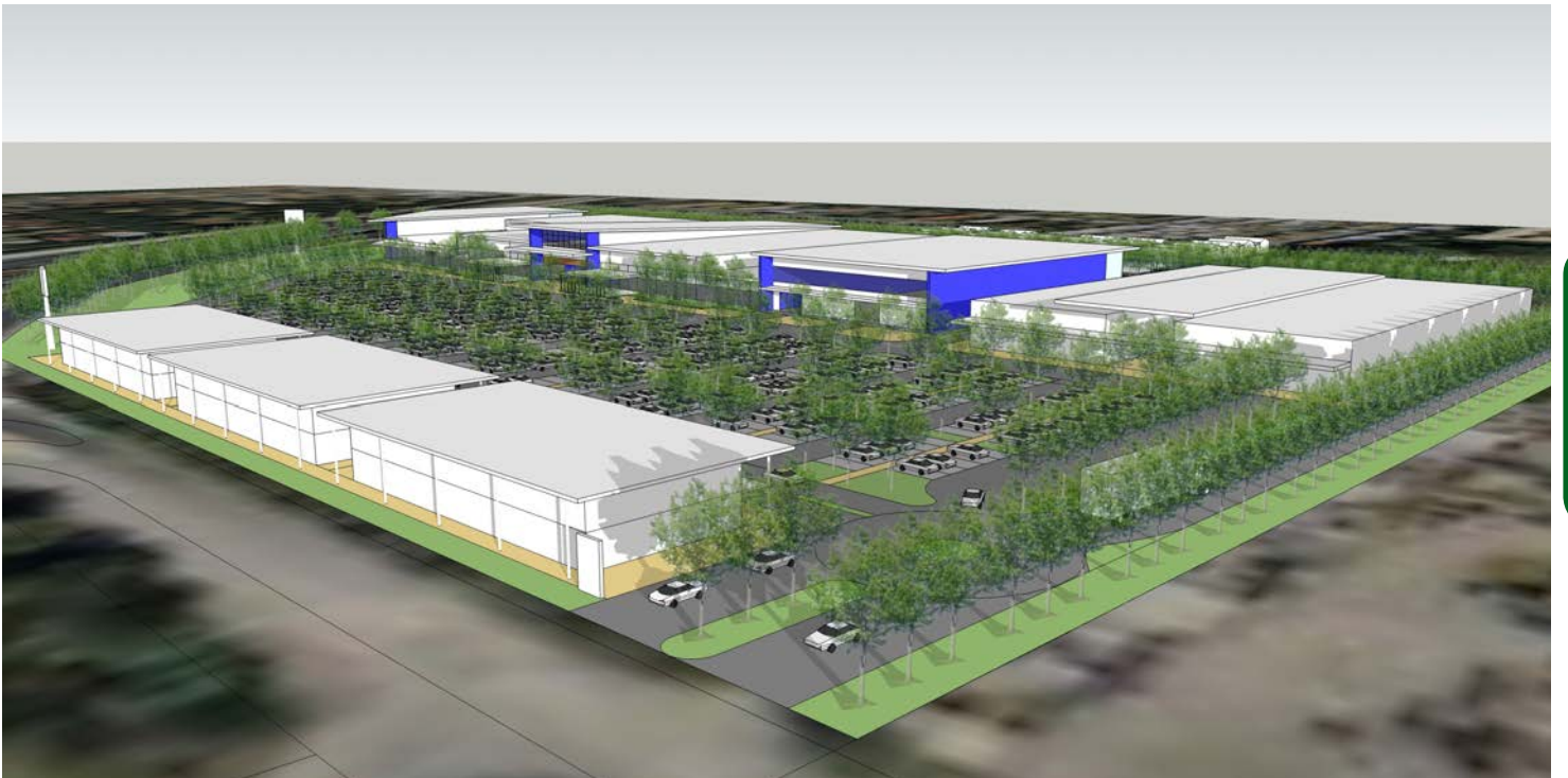
Figure 8.1.4 - Centralised car parking area and water sensitive urban design- A centralised landscaped car park area which adopts water sensitive urban design principles could serve all business park land uses. Given the amount of hardstand area that would be generated from required car parking numbers, this needs to be offset by a strong landscape plan with street trees and public domain and residue landscape area which would allow for some stormwater infiltration.
