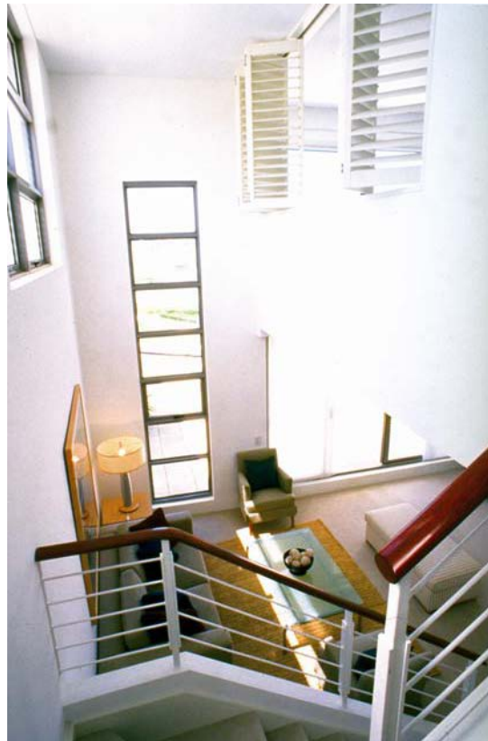
Double height ceiling spaces can significantly increase light penetration into narrow or one-sided apartments as well as add to the quality of the internal space.
