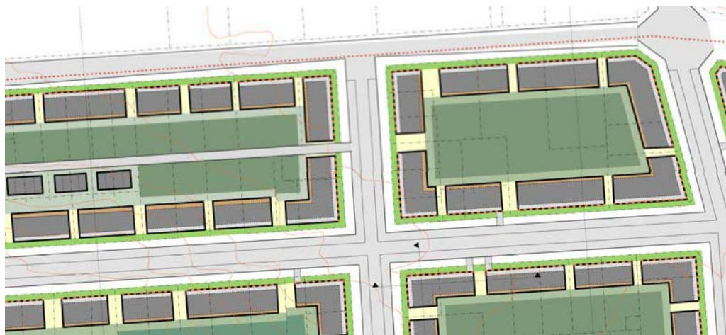
Illustrative block layout showing how the larger block edge developments define the street edge and relate to one another and create vegetation corridors to the rear of sites.
