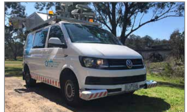
Urban roads in the Tweed will be tested using a Network Survey Vehicle (NSV) and will measure the road surface at a single pass.
