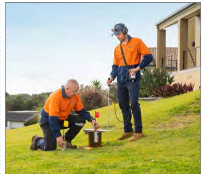
Technicians using the acoustic technology to detect water leaks.
