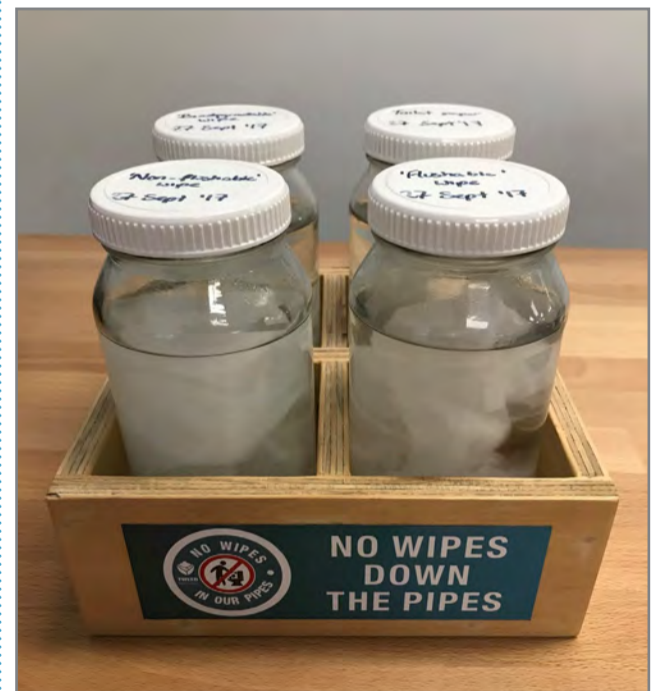
A Tweed Shire Council wet wipes experiment over 3 years has shown that wipes do not break down over time – imagine what they're doing in our sewer system.
