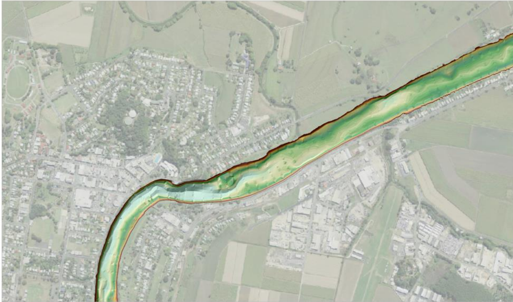
Image 4. Tweed River Bathymetry Model (After Tinning)
