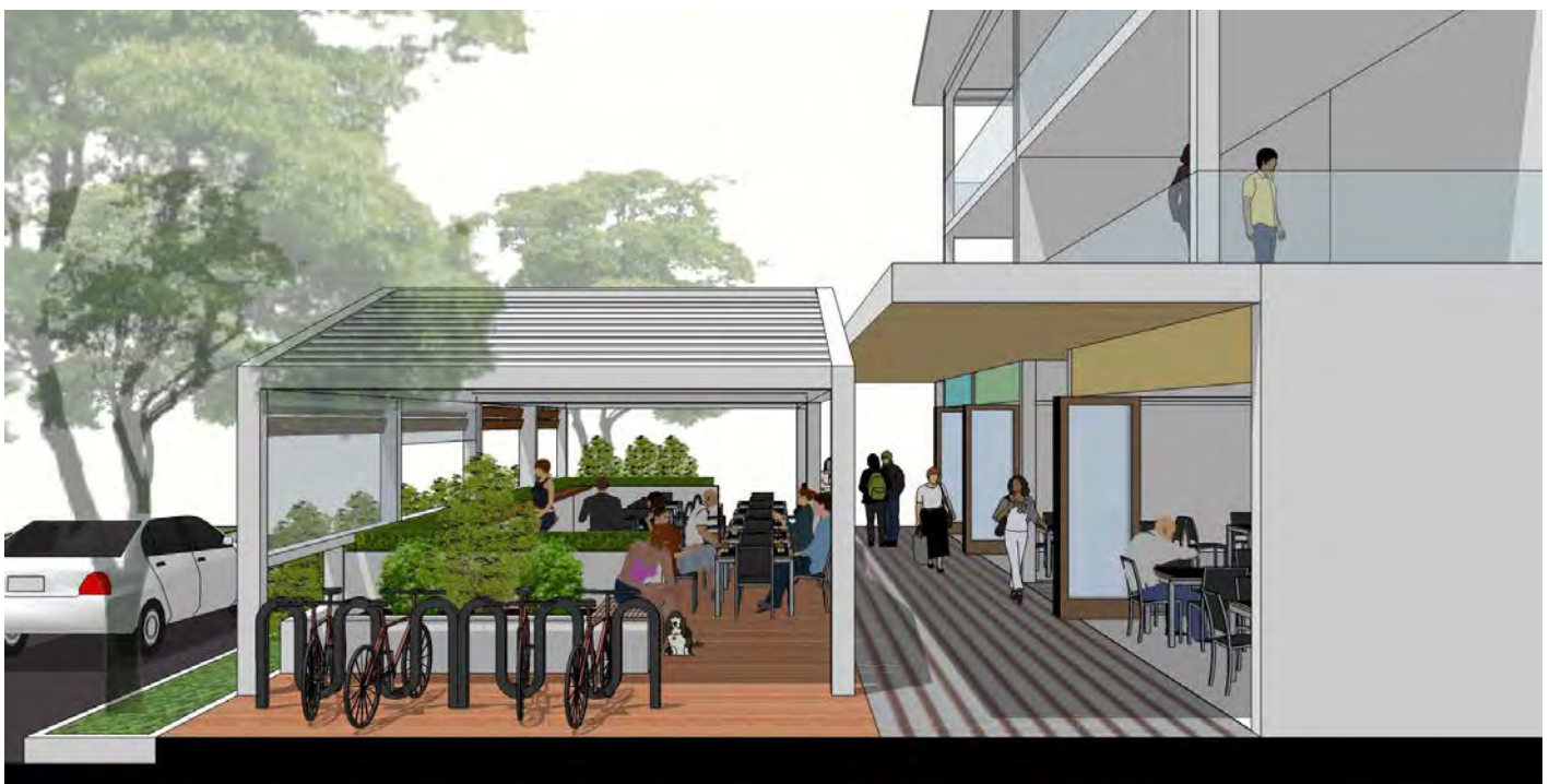
Figure 3.25 Outdoor dining areas – Design outdoor dining areas to achieve universal access and a balance between rain, wind and UV protection, shade and filtered light. Use a mix of marine tolerant materials and integrate landscaping, street furniture and bike parking.
