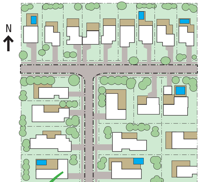
Grided road network results in rectilinear allotments with favourable north-south or east-west orientation which are easier to design to and build on.
