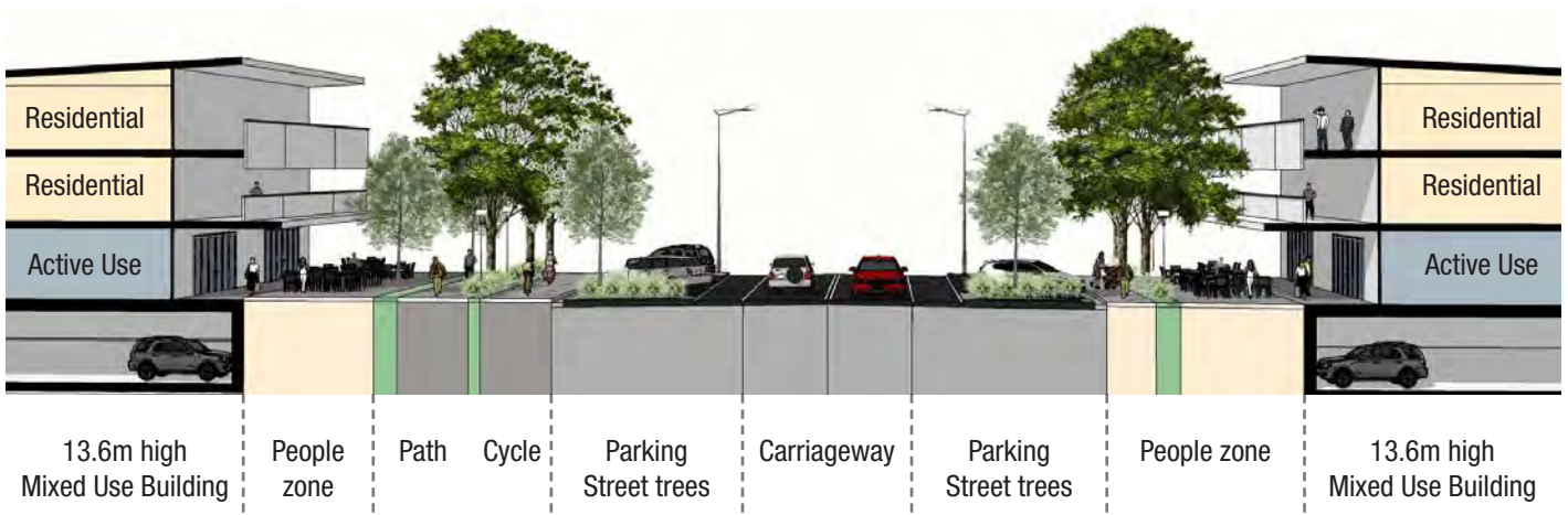
Figure 8.11 Indicative Turnock Street Section – Mixed Use Interface
