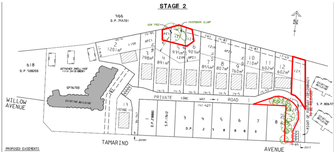
Proposed Site Plan highlighting areas to be protected under an 88B Restrictive Covenant ('Z' or red denotes area to be protected).
