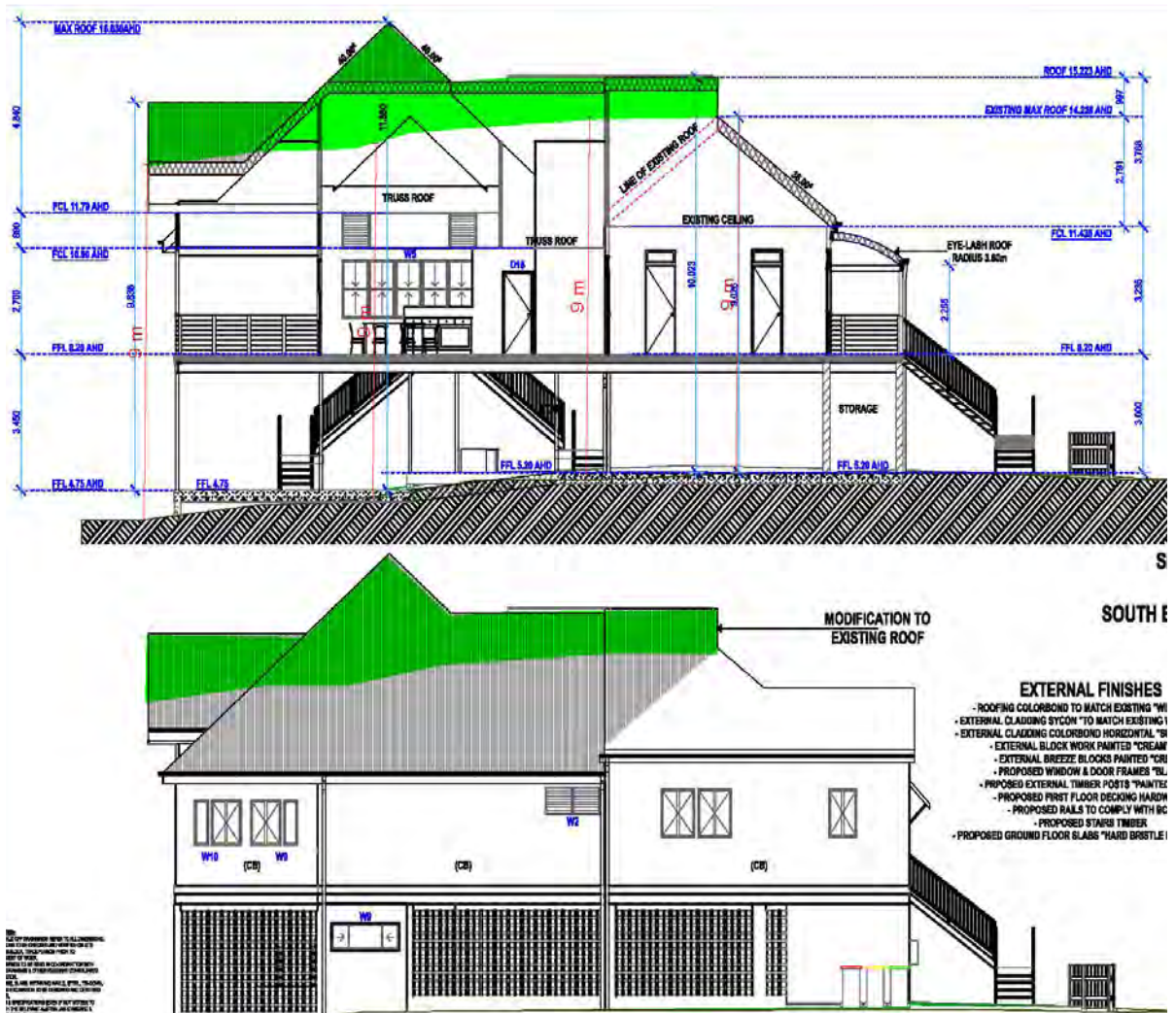
Figure 1 – Portion of the already constructed roof above the 9m height limit.
