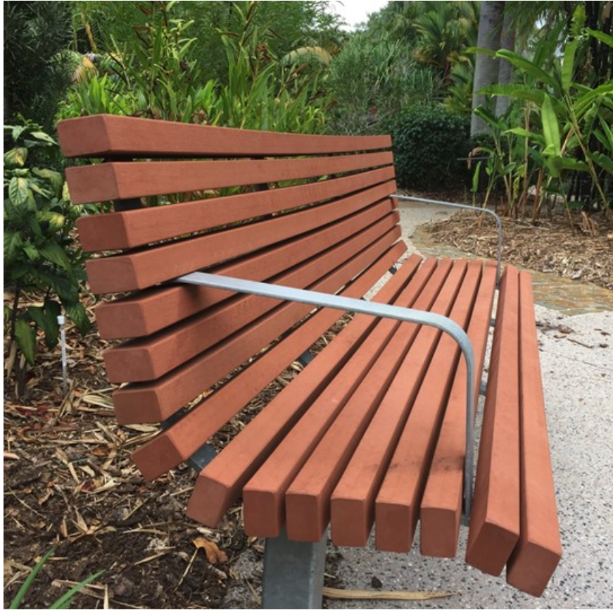
Figure 2: Solid recycled plastic battens showing sagging between frame connections
