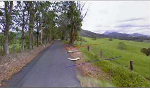
Figure 4 Red line = existing access location for proposed Lot 13 Blue line = alternate location to avoid the need to remove the large existing gum tree.
