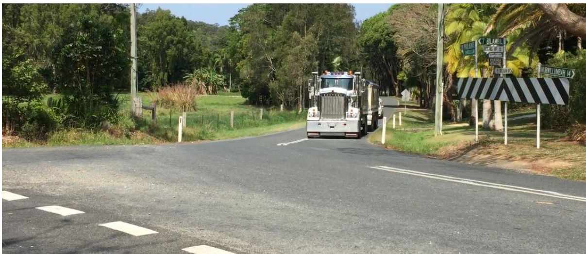
Site 5 Hogan Road Intersection: PBS vehicle travelling westbound on Dulguigan Road - Wheels just remained within the westbound travel lane when negotiating the left hand curve
