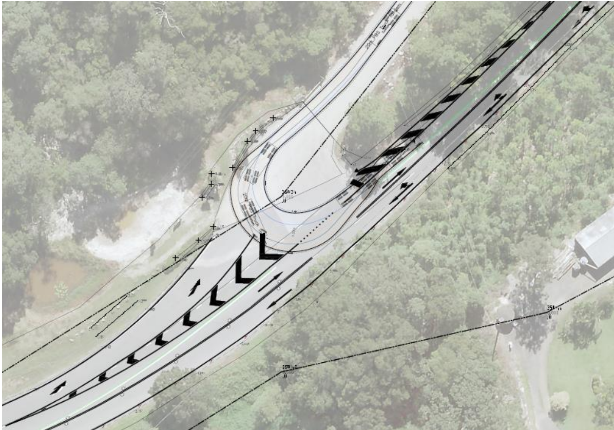
Figure 3.1: Portion of Preliminary Sketch titled "Turns - 20m PBS Vehicle, Quarry Entrance"
