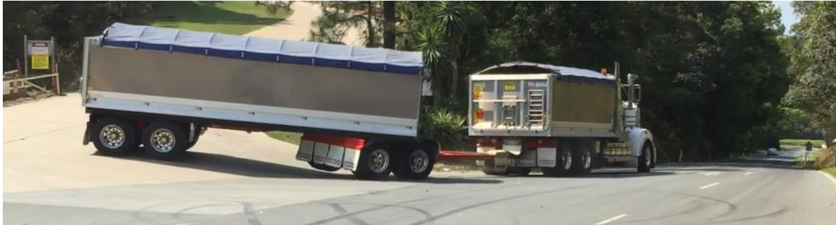
Site 1 Quarry entrance: PBS vehicle exiting quarry and turning left (eastbound) onto Dulguigan Road - Wheels just remained within the eastbound travel lane
