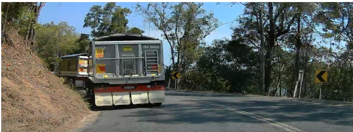
Site 3 First Curve East of Mayes Hill Road: PBS vehicle travelling eastbound on Dulguigan Road - Rear wheels travelled slightly off the sealed road surface when negotiating the left hand curve
