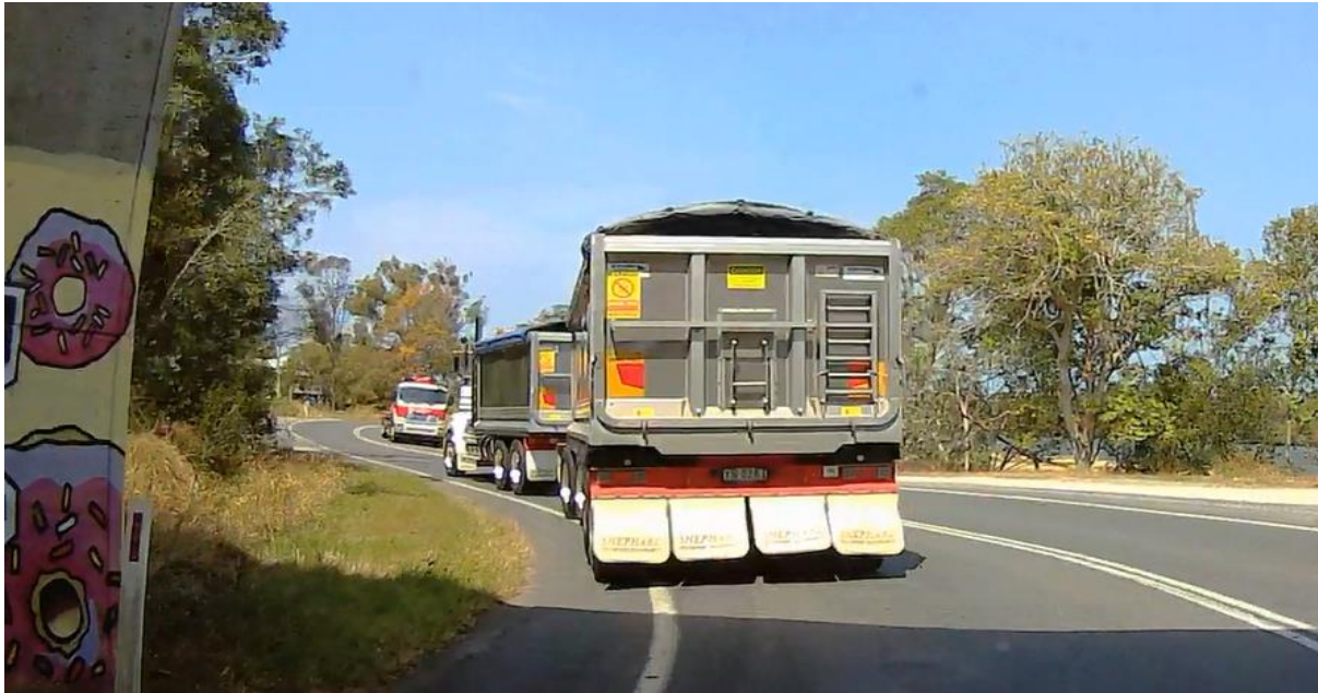
Site 4 Under Terranora Road Structure: PBS vehicle travelling eastbound on Dulguigan Road - Two sets of rear wheels travelled outside of road edge line when negotiating the left hand curve, however wheels remained on the sealed road surface
