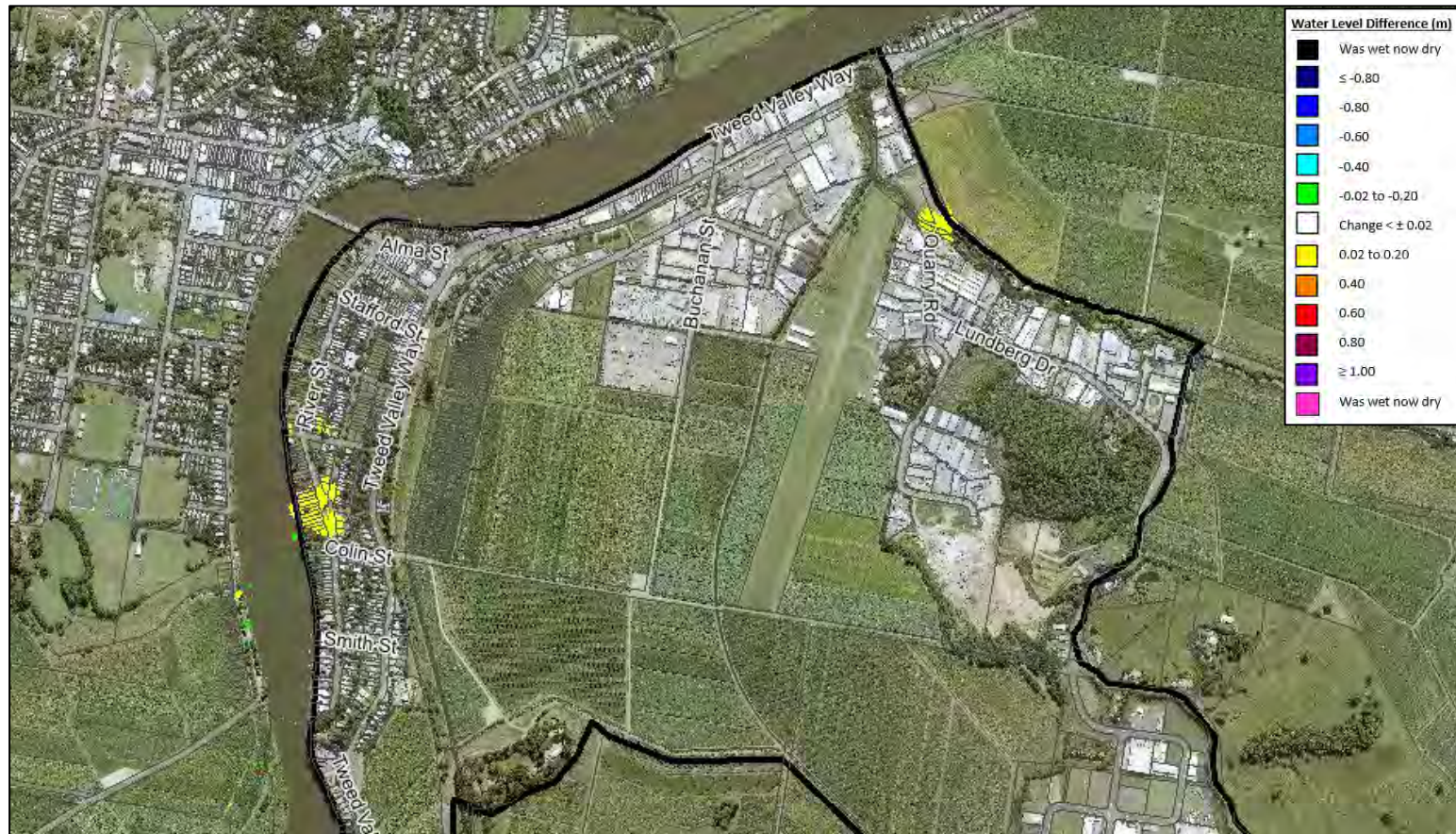
Plate F2 1% AEP Flood level difference map with failure of the South Murwillumbah levee
