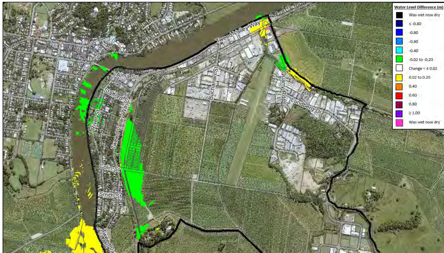
Plate F5 1% AEP Flood level difference map with blockage of all hydraulic structures except Murwillumbah Bridge
