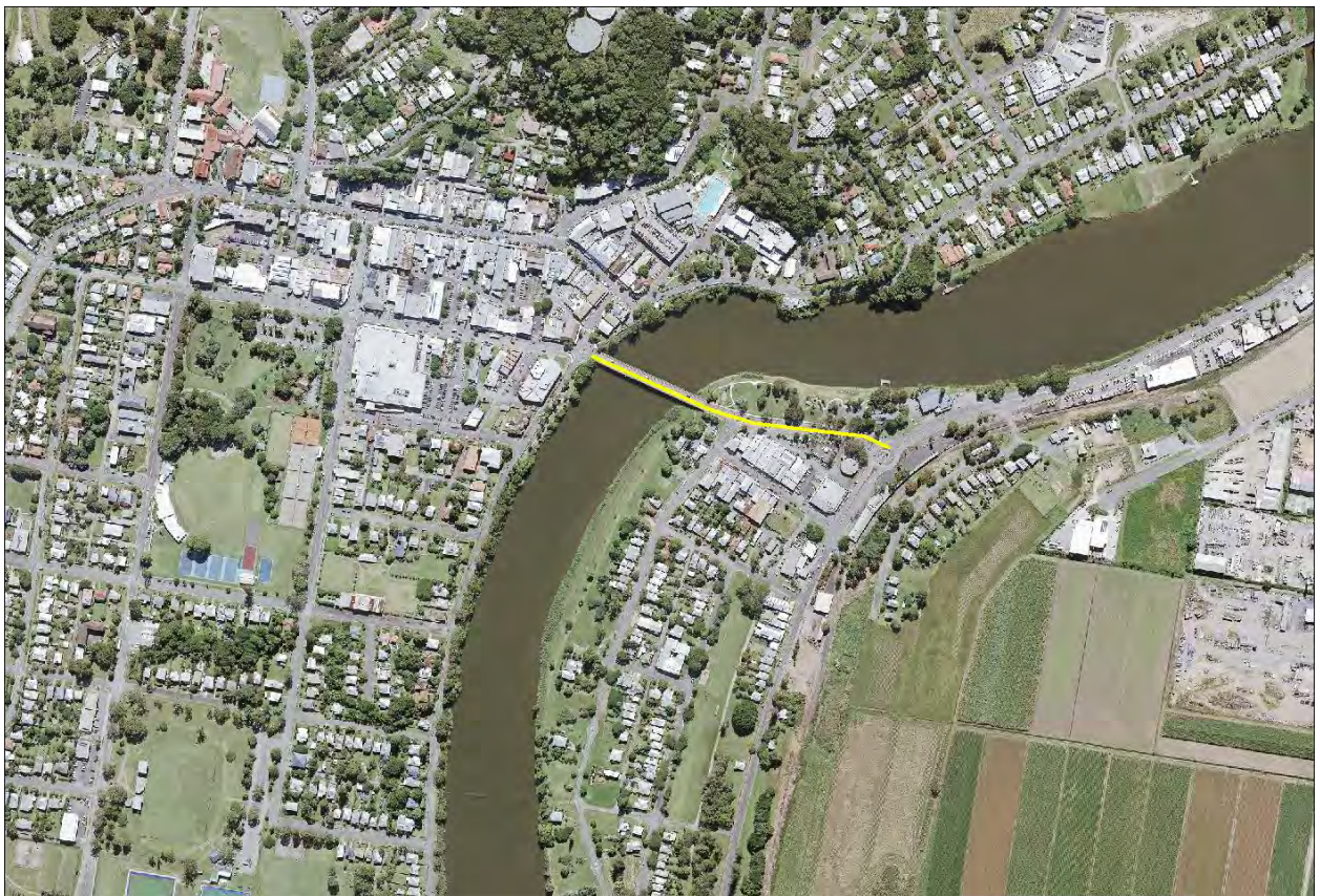
Plate 4 Extent of cross-section (yellow) used to derive synthetic Murwillumbah rating curve for current study
