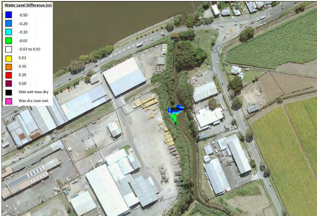
Plate 44 20% AEP Flood Level Difference Map for High Level Condong Creek Outlet (FM17)
