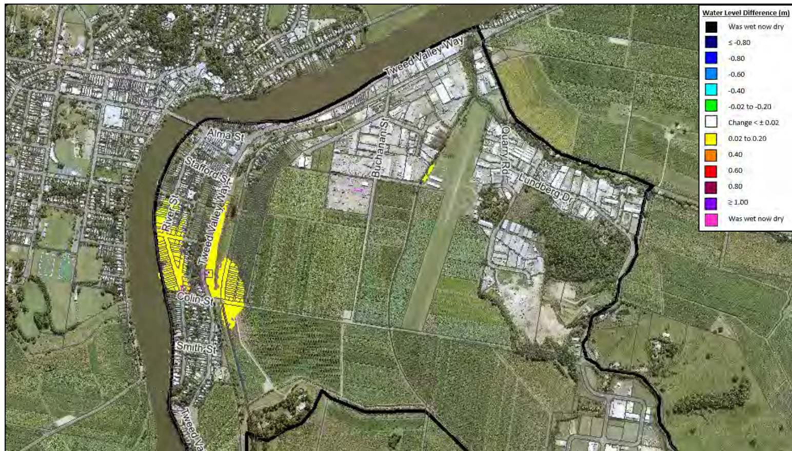
Plate F1 20% AEP Flood level difference map with failure of the South Murwillumbah levee
