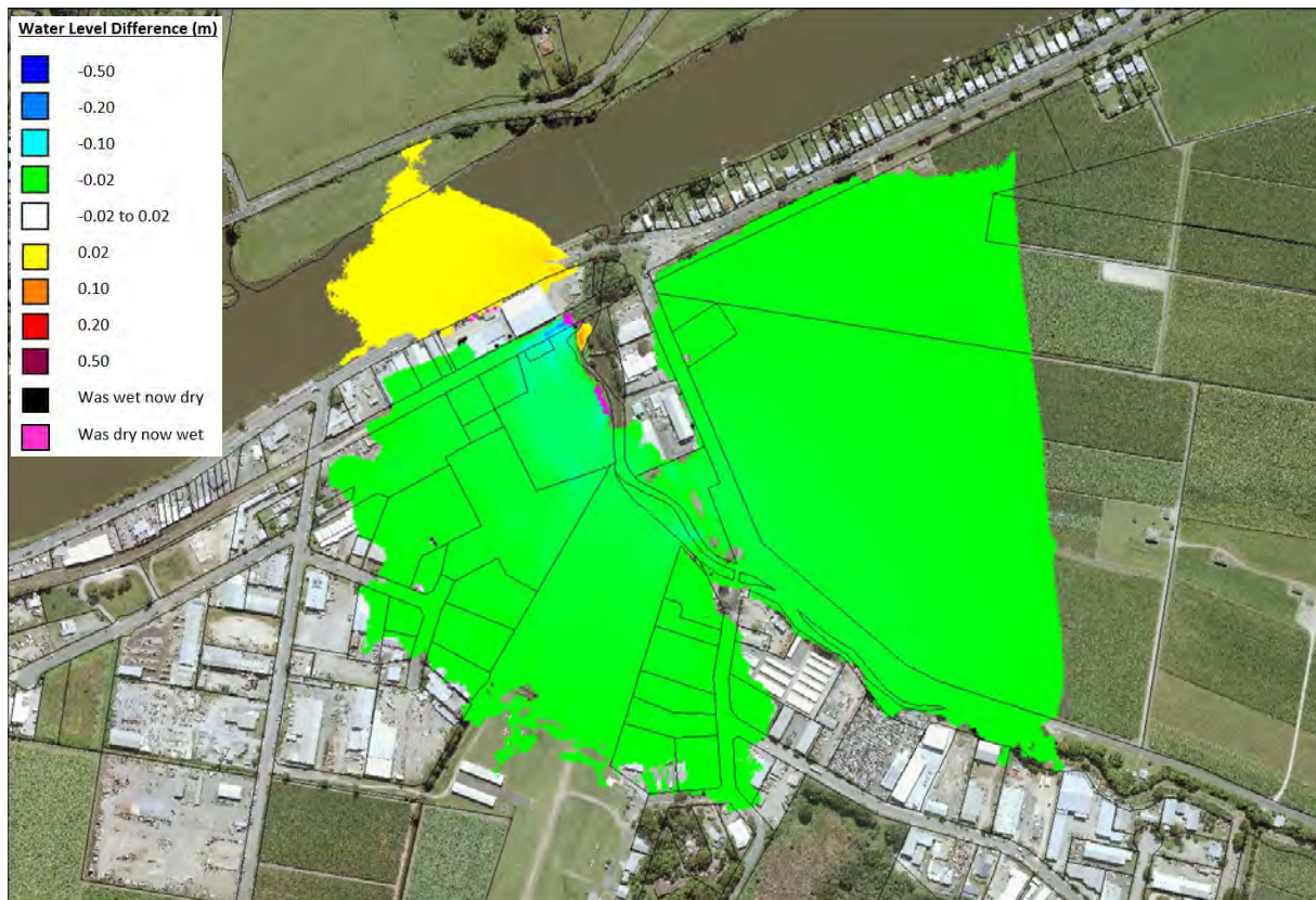
Plate 43 1% AEP Flood Level Difference Map for Condong Creek High Flow Bench (FM16)
