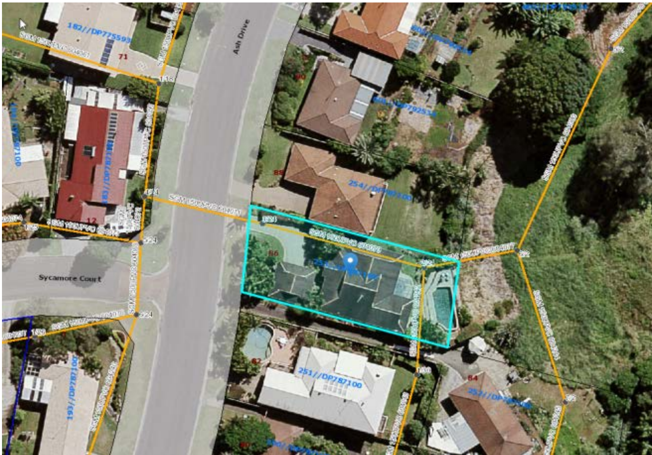
Figure 3 - showing the sewer gravity mains within Lot 253
