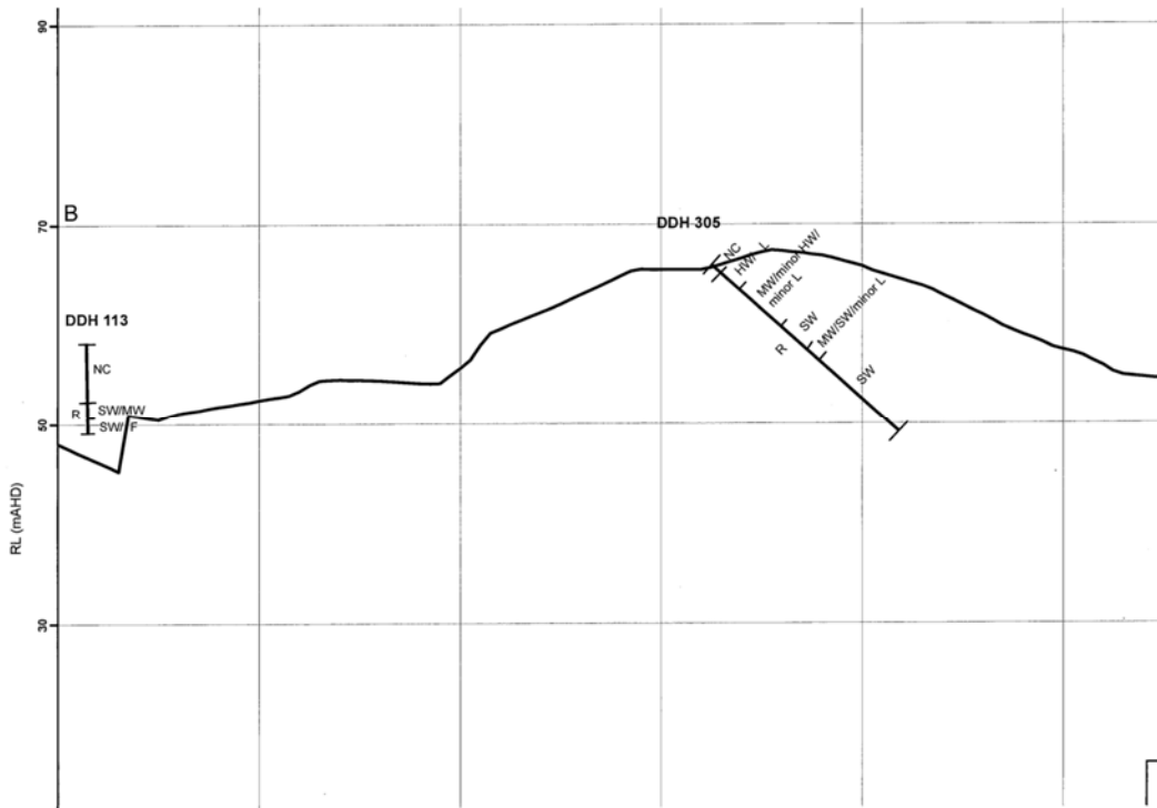
Figure 5-4: Section B Spillway Alignment Interpreted Geology
