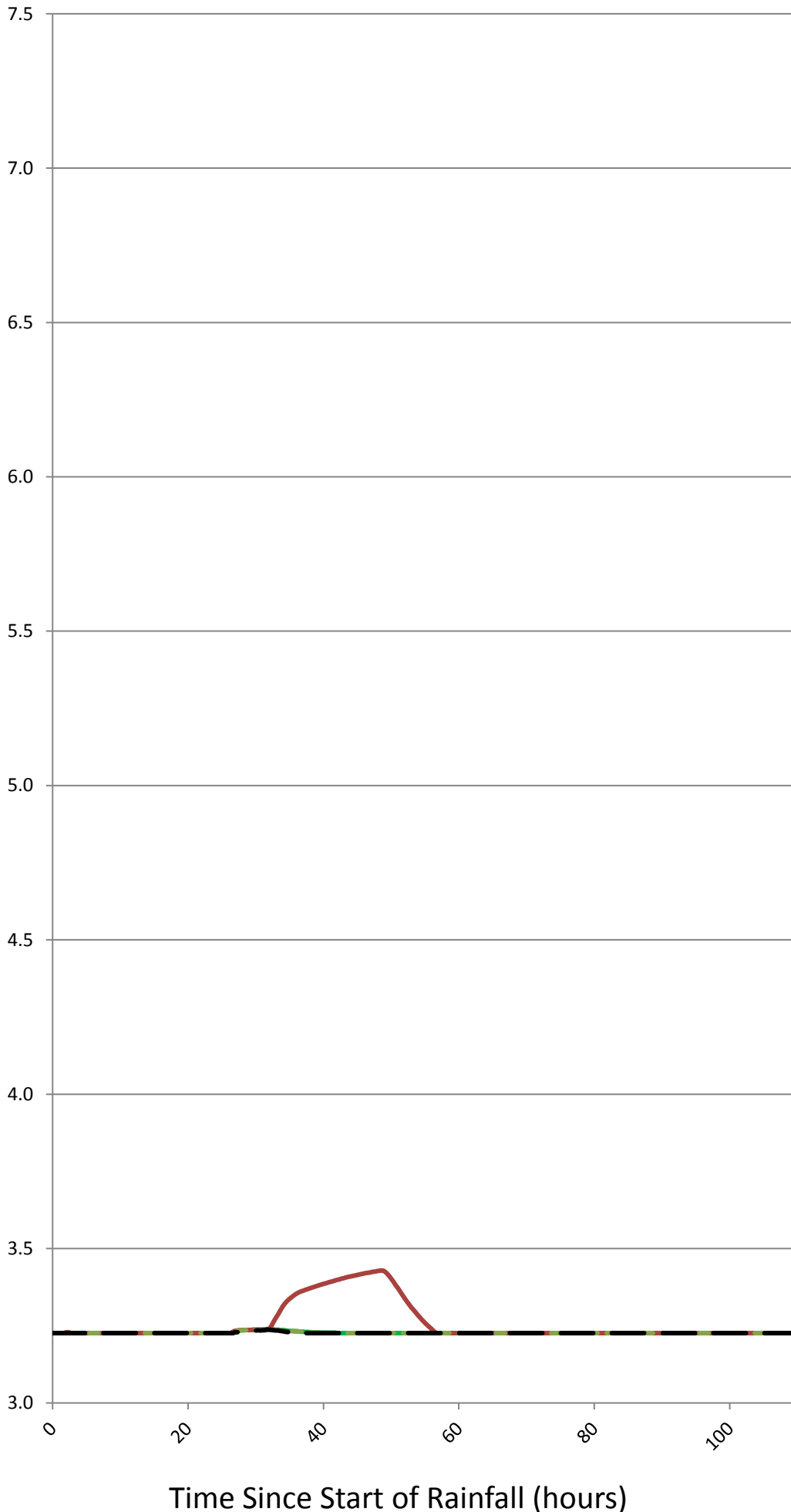
Figure K3.2: 5%AEP Stage Hydrograph Comparison on Wollumbin St at Knox Park
