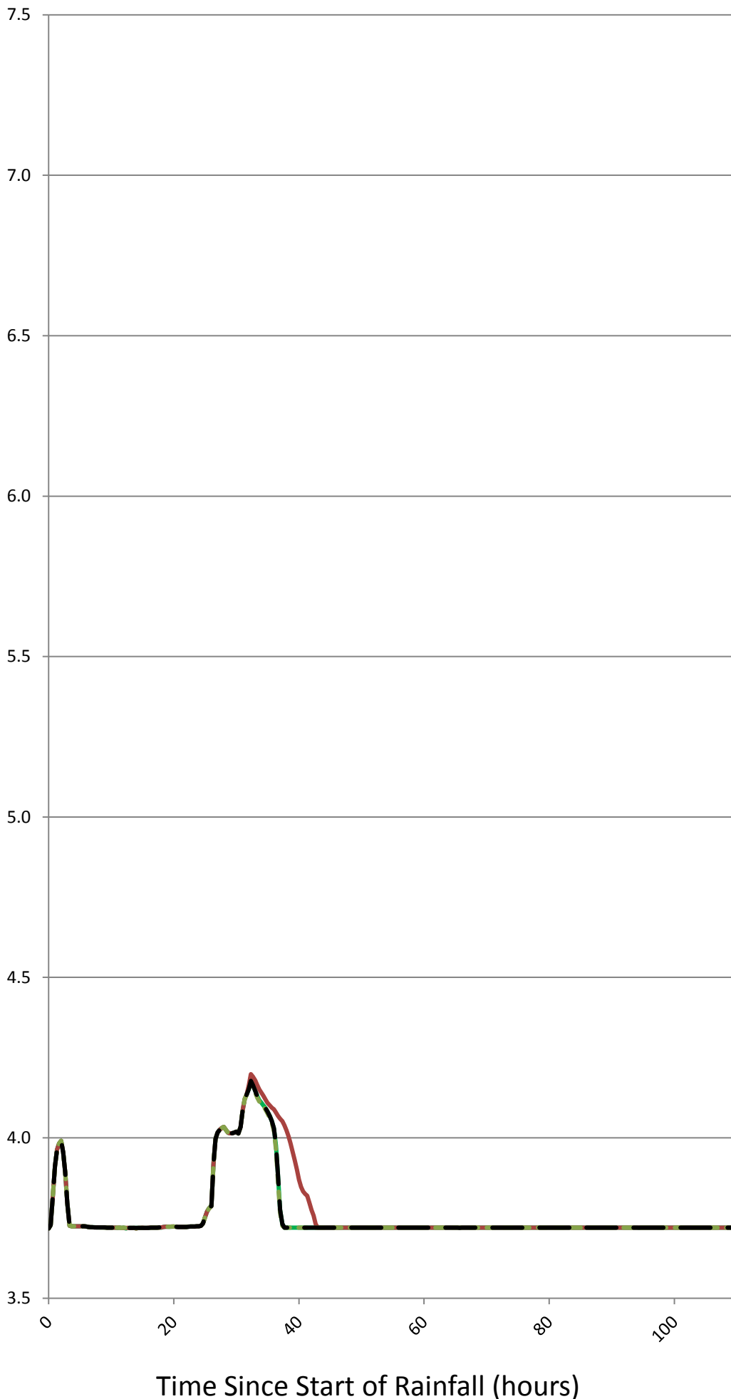
Figure K4.1: 20%AEP Stage Hydrograph Comparison at Murwillumbah CBD
