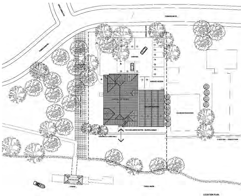
Figure 4 Site plan. The drawing shows the existing buildings, parking and access and river pontoon. A tone on the plan indicates the presumed location of the former Ferry Wharf access road (Refer Figure 6).
