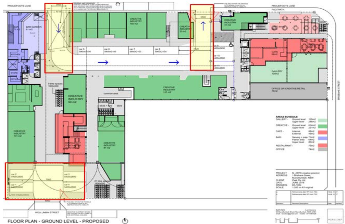
Figure 5: Proposed Ground Level Plan demonstrating vehicular access to the site
