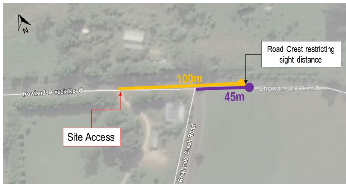
Figure 2.1: East Facing Sight Distance
