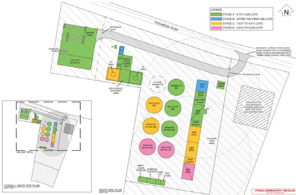
Figure 3: WWTP Staging Plan
