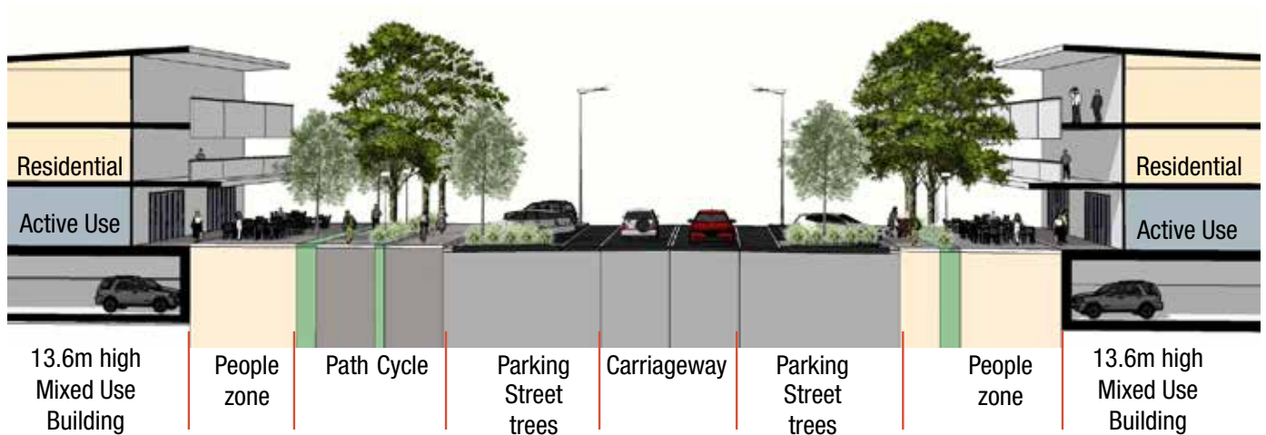
Figure 2.18 - Indicative Turnock Street Section - Mixed Use Interface
