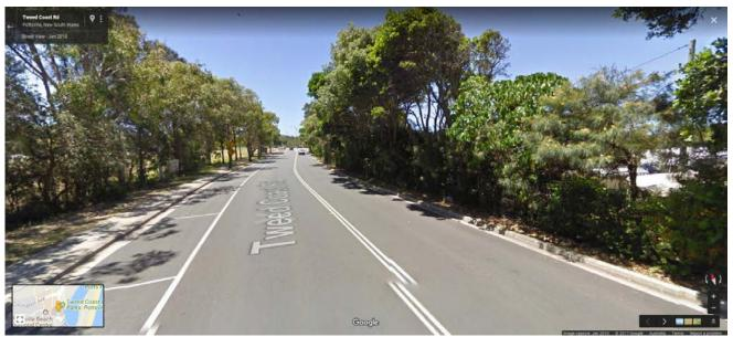
Google Maps view looking north along Tweed Coast Road from Phillip Street (Overall Drive). Additional parking spaces proposed for the east side of the road. Double centre line to be relocated to reduce traffic lanes to a width of 3.3 metres.
