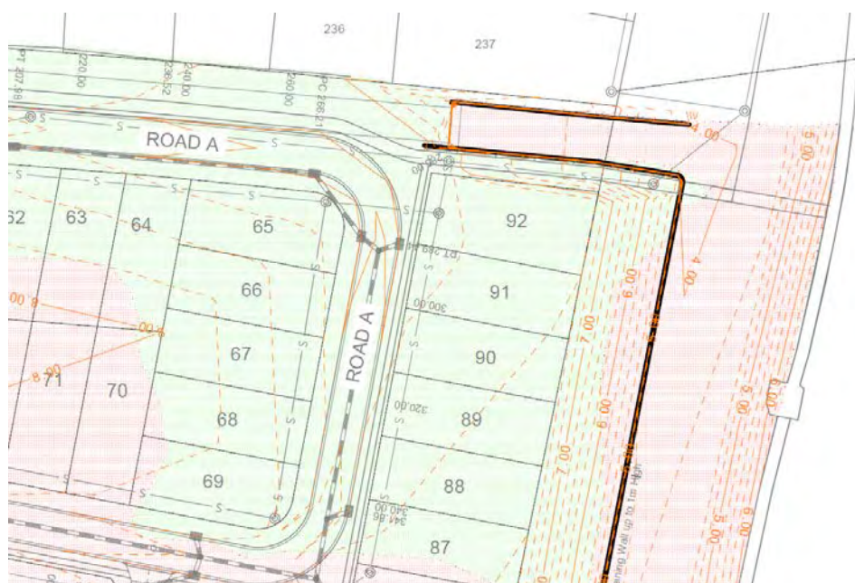
Figure 9: Extract from Bulk Earthworks Plan (demonstrating retaining walls to north east corner of site)
