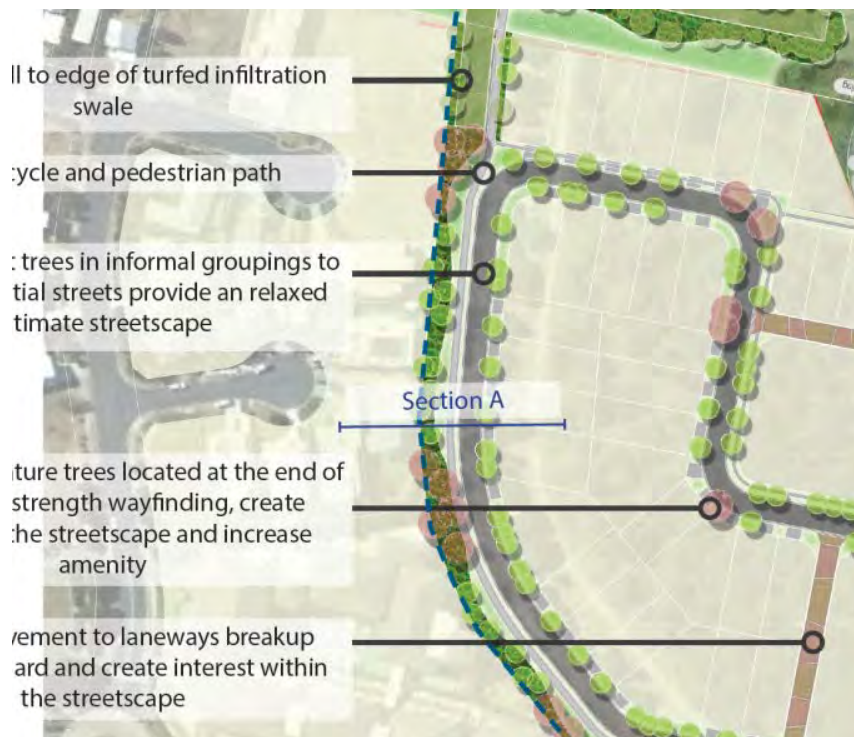
Figure 14: North Boundary Treatment with road
