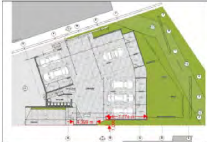
Figure 2: Image illustrating garage level walls within side boundary setback
