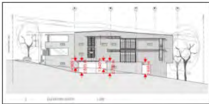
Figure 3: Image illustrating garage level walls within side boundary setback
