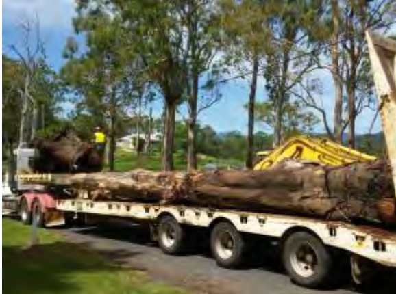
Hardwood logs and root balls will be used to stabilise banks on the Oxley River and provide habitat for a range of aquatic and terrestrial species.
