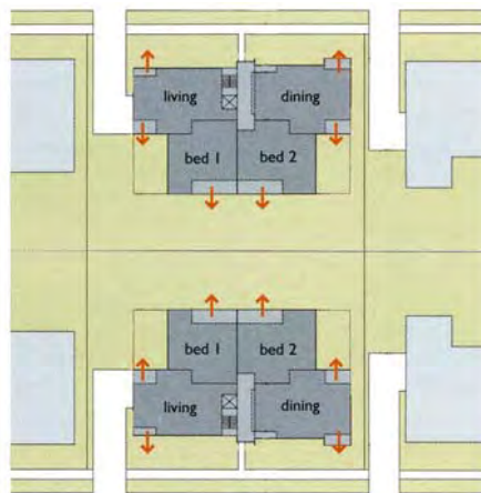
Living rooms and external living areas can be oriented to the front and rear of the site.
