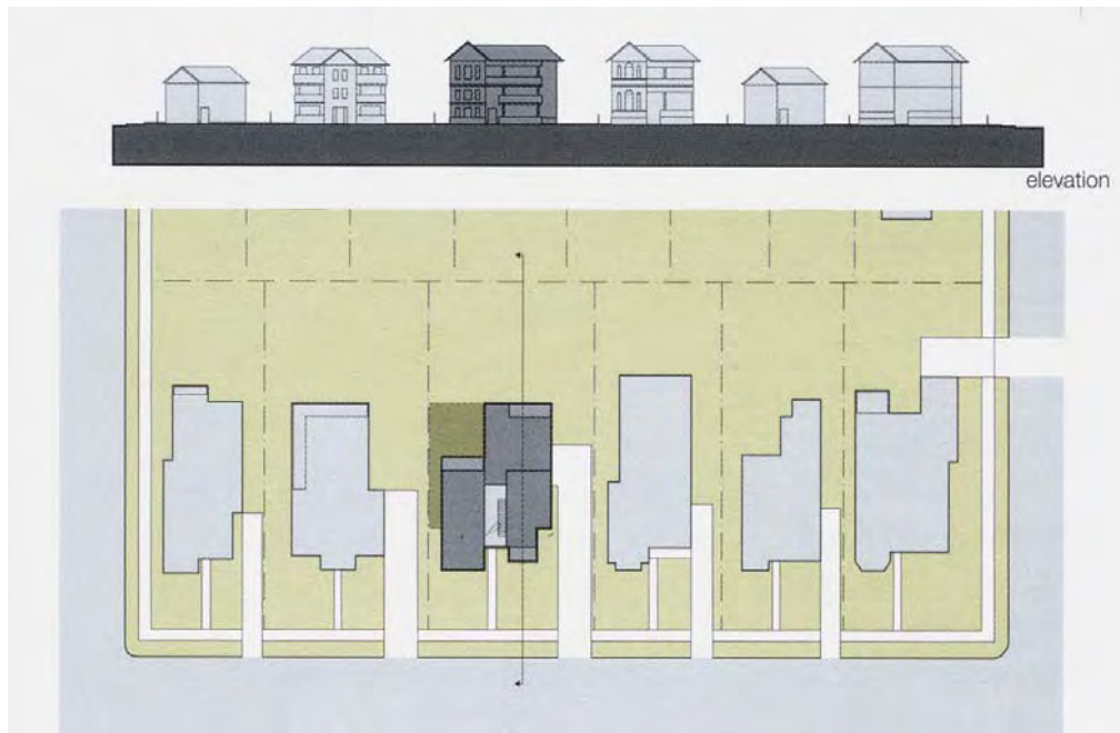
Illustrative elevation and street plan of the small residential flat building type (Image from the Residential Flat Design Code).
