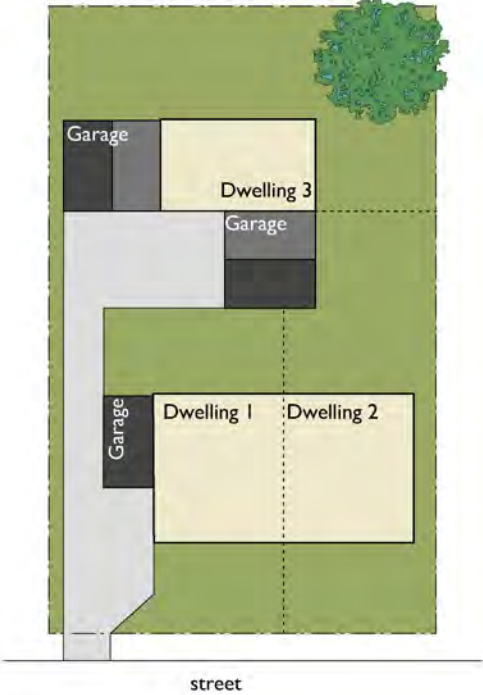
Illustrative site layout of Town Housing, on a small lot with three dwellings.
