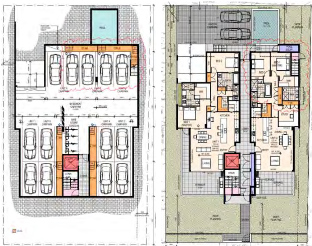
Basement and ground level car parking configuration
