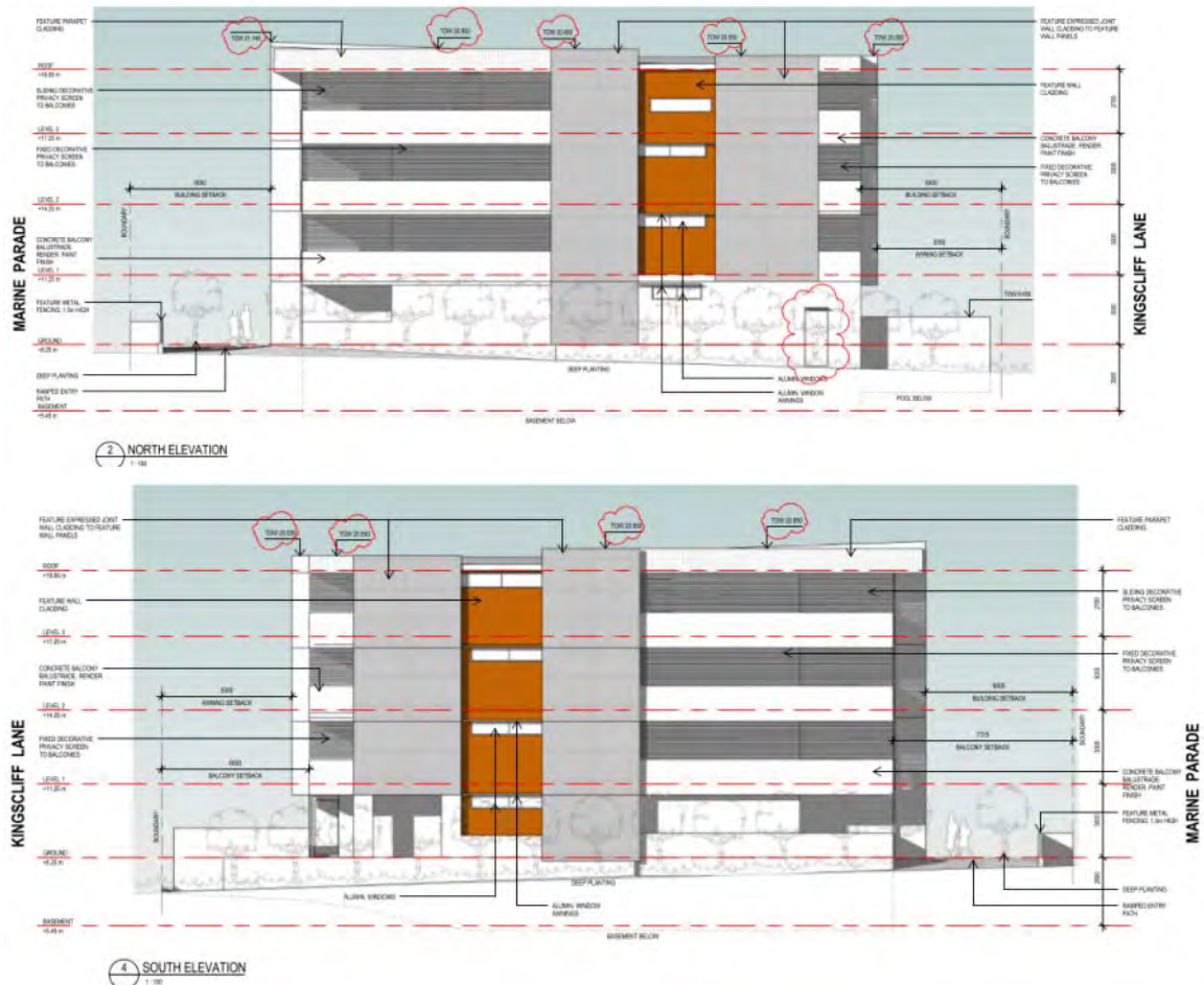
North and South elevations showing the lack of windows and balconies with extensive privacy screening.
