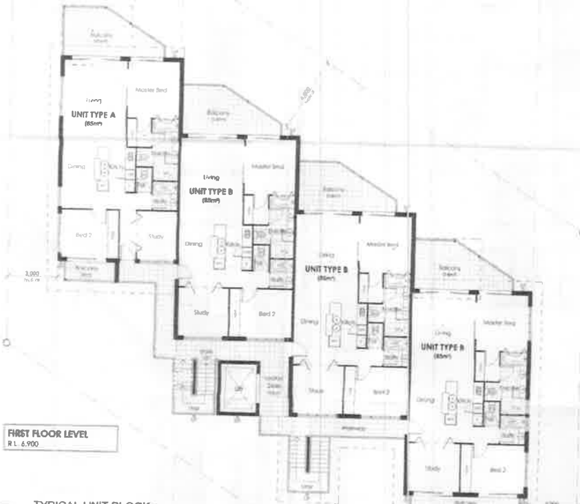
P1 TYPICAL UNIT BLOCK - FIRST FLOOR PLAN SCALE 1:100
