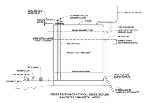
Note: To be considered as an above ground rainwater tank, the outlet of the overflow fitting must be a minimum of 375mm above the 1 in 100 year flood level.
