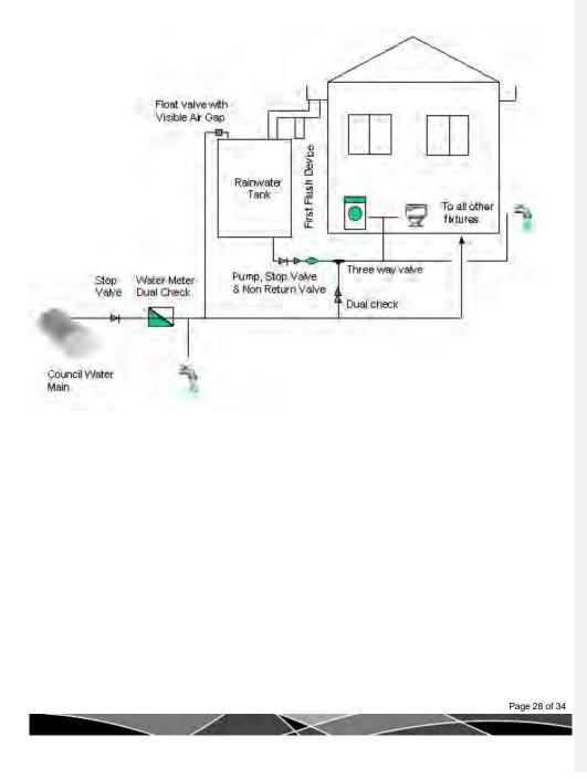
Above Ground Tank with Air Gap (Indirect Town Water Interconnection)
