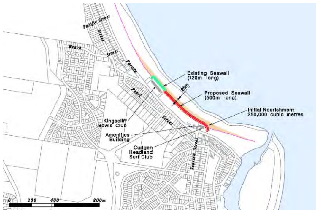
Figure 3-4 Terminal Protection with Beach Nourishment Option as Proposed in Umwelt (2005a)
