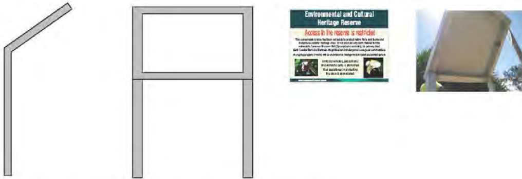
50mm aluminium frame 600mm x 600mm - 1.5m high $270 installed, anti graffiti covering
